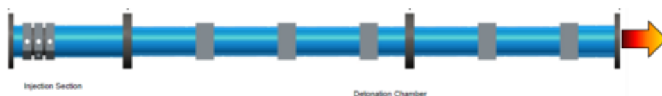
Figure 63. Schematic diagram of PDE
