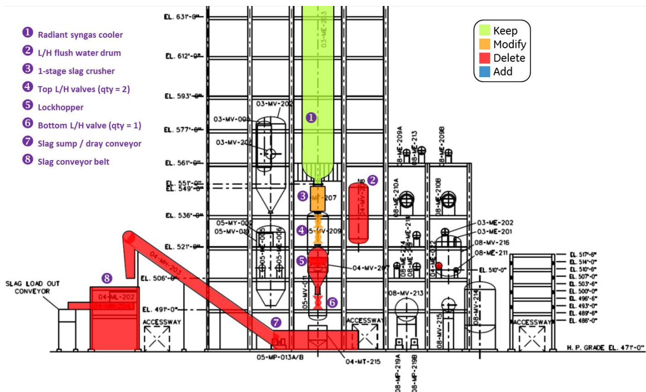
Figure 132. Gasifier Support Structure Required for Lockhopper System
