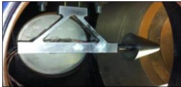
Figure 111. Instrumented blunt nose cone pitot used for total pressure measurement.
