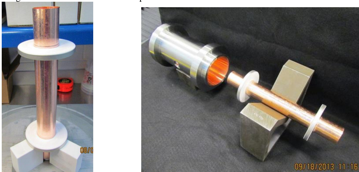
Figure 9: Windows and Inner Conductor sub-assembly (on the left) and both Coupler sub-assemblies (on the right).
