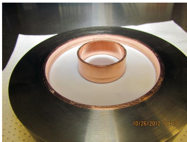
Figure 4: A coaxial window assembly made with an explosion bonded Compression Ring. For scale, the window ceramic OD is approximately 3 inches.
