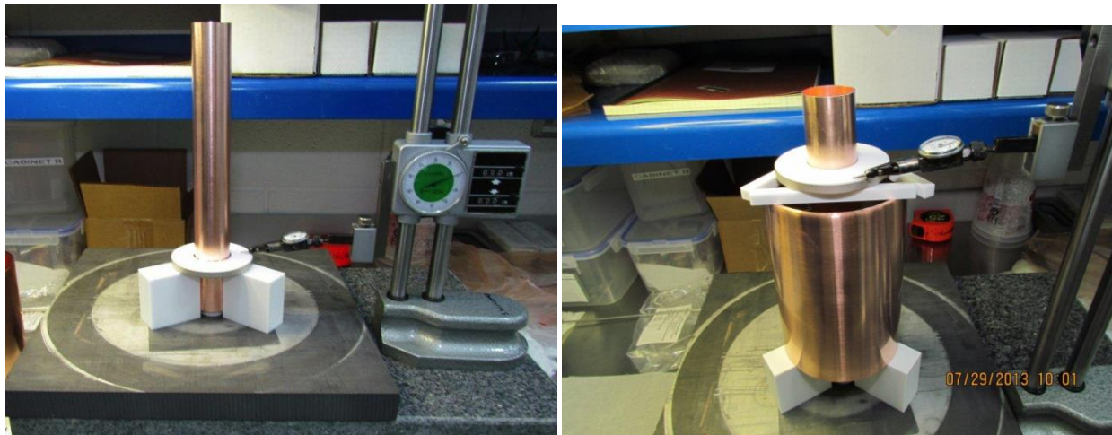
Figure 8: shown are some of the steps of for the Dual Window / Inner Conductor braze stack.
