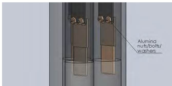
Fig. 41: Illustration of the electrical isolation of samples using alumina nuts/bolts/washers.
