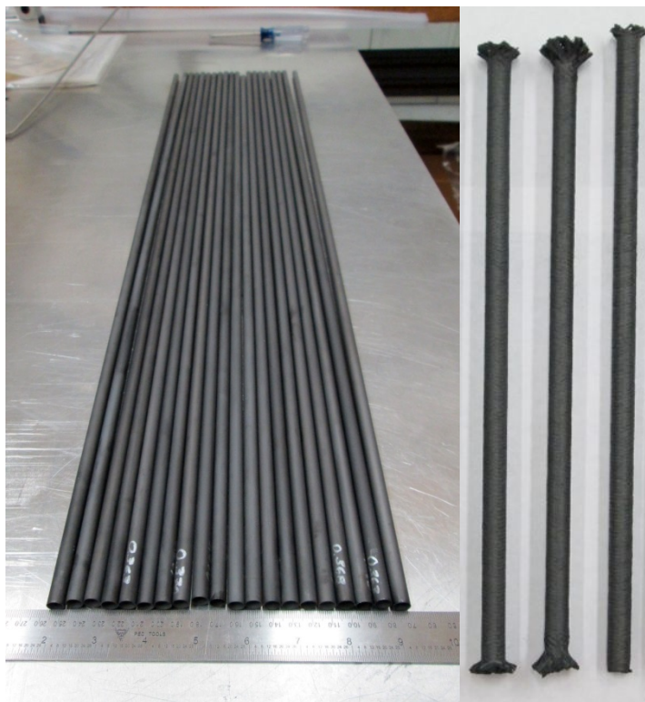
Figure 24: (left) as-received thin-walled Hexoloy SiC tubing, (right) inner monolith structure following fiber preforming and initial infiltration
