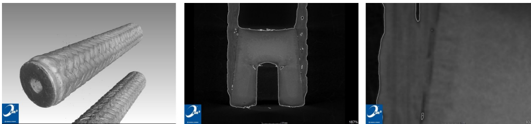
Figure 99: XCT scan of typical GA-TC3-I-X sample, showing good endplug density and alignment
