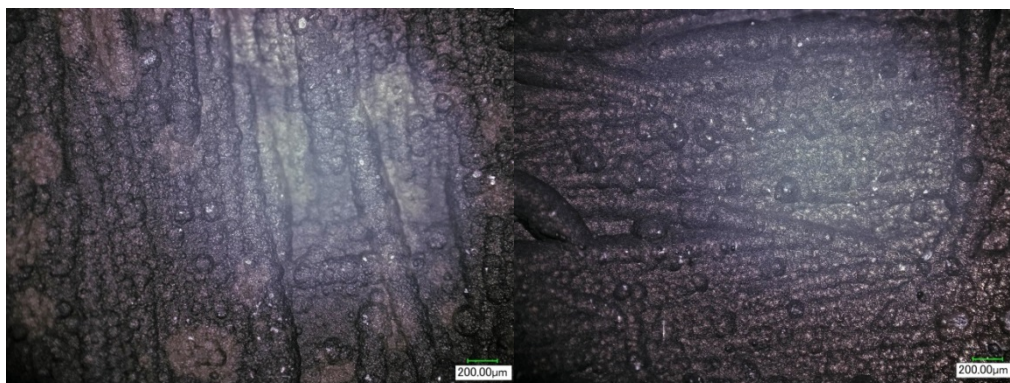
Figure 61: Surface discoloration observed for SiC-SiC samples exposed to autoclave testing
