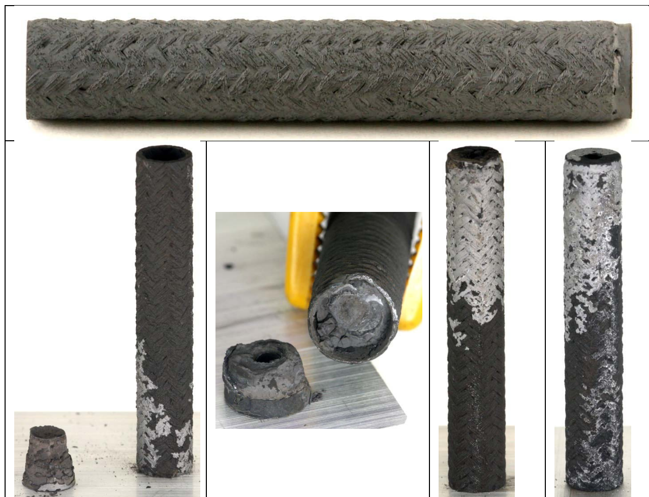
Figure 7. Photographs of GA end-sealed tubes: above - GA1-TCJ-I-1 unirradiated, below – after Stage 2 irradiation, left to right, GA1-TCJ-I-1 (end cap separated completely from tube during capsule disassembly), GA1-TCJ-I-6 (end cap broke at bottom of mounting hole but lower section remained bonded to tube), GA1-TCJ-I-2, GA1-TCJ-I-3. Note that the end caps remained bonded for samples 2, 3, 4, 5, 7, and 8.
