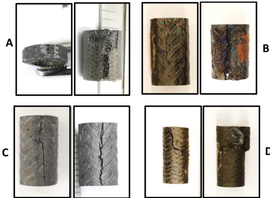
Figure 54: Comparison of cracking behavior between pairs of oxidized samples (left half of paired pictures) and as-received samples (right half of paired pictures)
