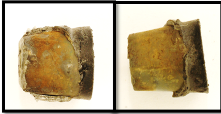
Figure 35: Endplug joint failure comparison for GACE-A and GACE-B series
