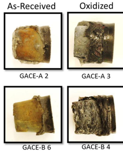
Figure 55: Endplug joint failure comparison for GACE-A and GACE-B series
