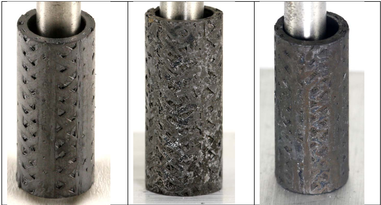
Figure 5. Photographs of GA3 tubes: left to right GA3-01 unirradiated, GA3-01 after Stage 1 exposure and GA3-05 after Stage 1 and Stage 2 exposure.
