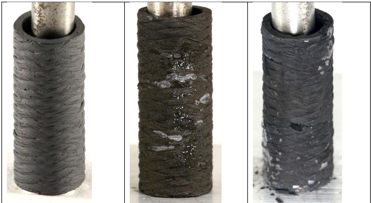
Figure 4. Photographs of GA2 tubes: left to right GA2-01 unirradiated, GA2-01 after Stage 1 exposure and GA2-08 after Stage 1 and Stage 2 exposure.
