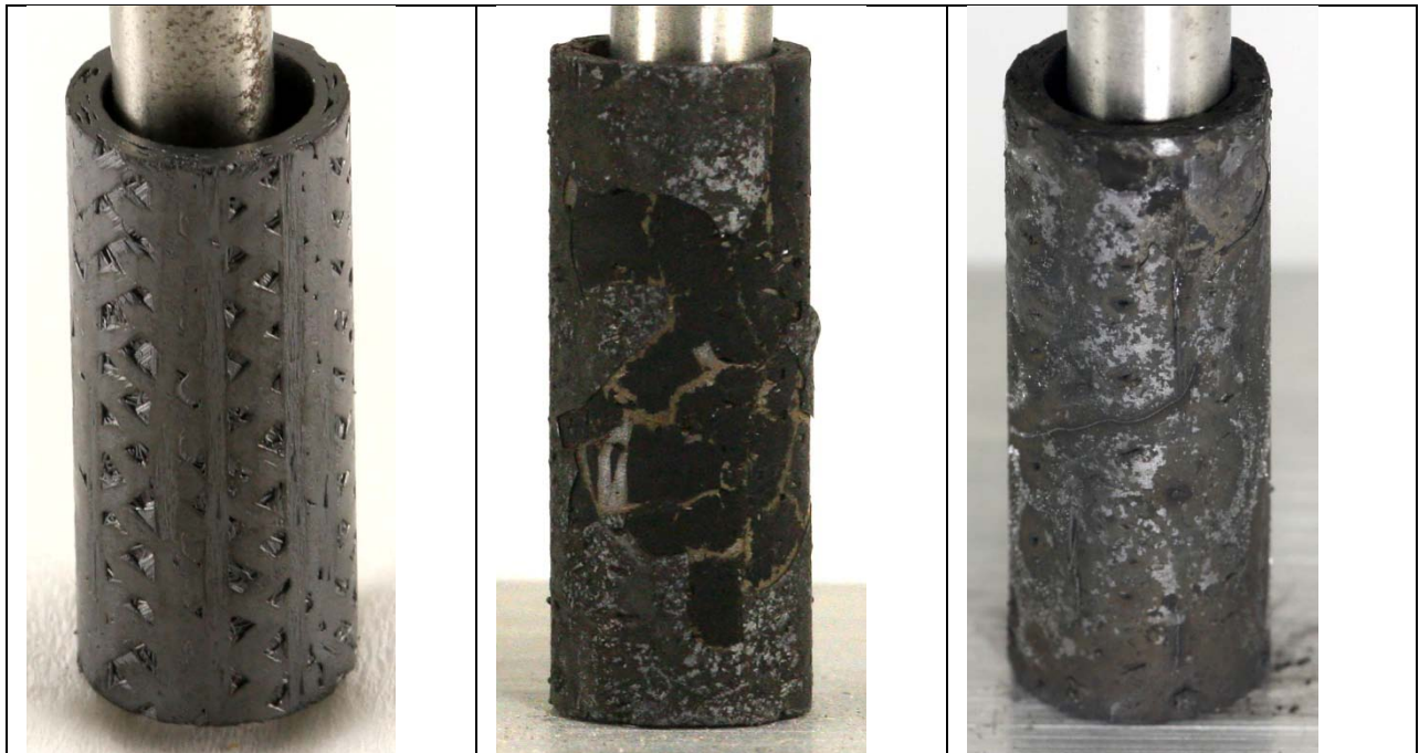
Figure 3. Photographs of GA1 tubes: left to right GA1-01 unirradiated, GA1-01 after Stage 1 exposure and GA1-?? after Stage 1 and Stage 2 exposure.
