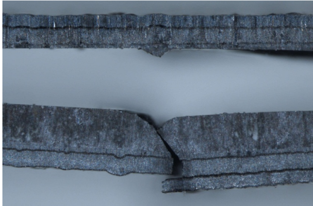
Figure 22: Four-point bend sample showing multilayer specimen with upper layers remaining intact while lower layers fractured.
