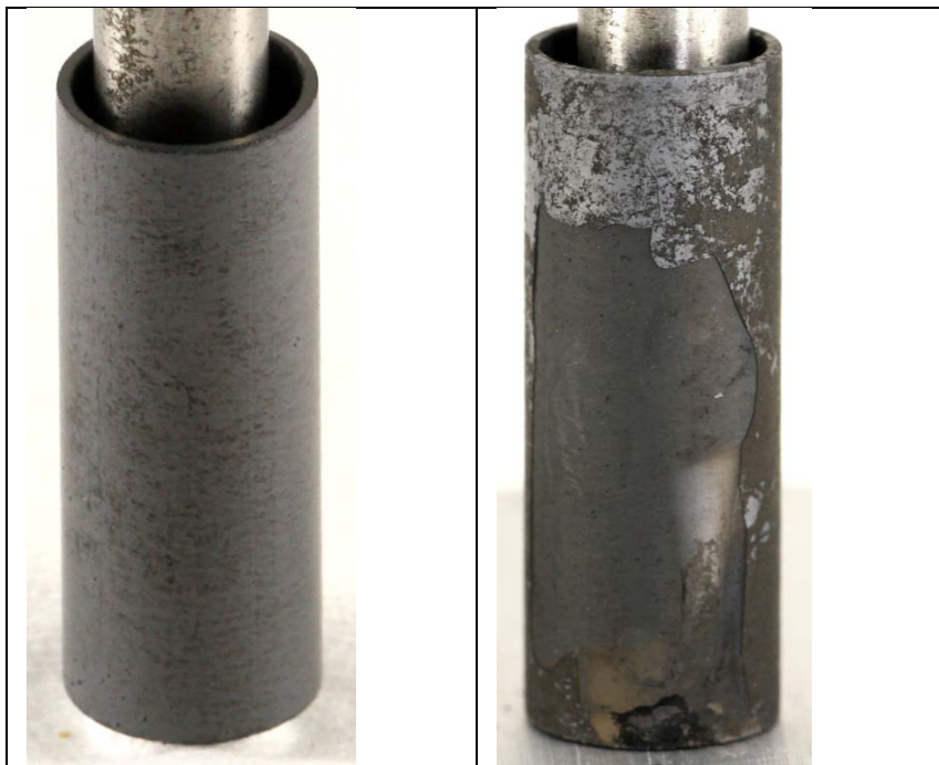
Figure 6. Photographs of GA4 tubes: GA4-01 unirradiated and GA4-01 after Stage 1 exposure.
