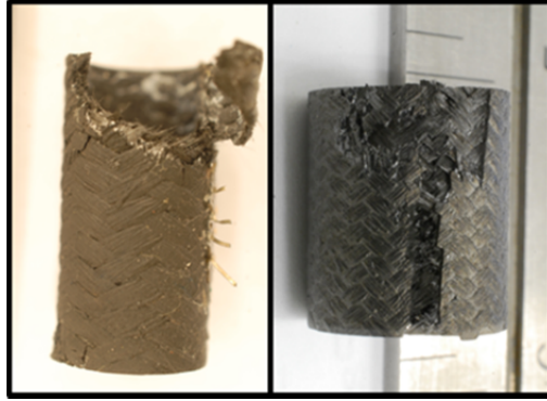
Figure 17: Comparison of Failure Characteristics of GAOE 2 (left) and 196.1.27 (right)
