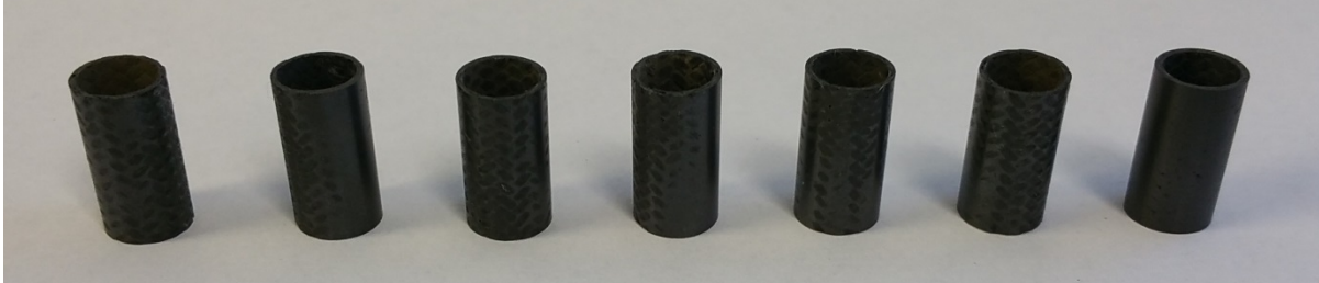
Figure 44: Seven polished tube samples prepared for analysis of roundness and wall thickness variation
