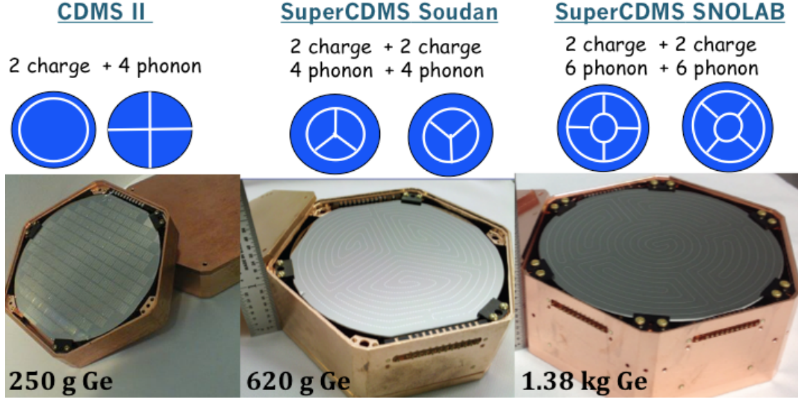
Figure 19: Detector configurations for the three CDMS experiments discussed in this proposal.
