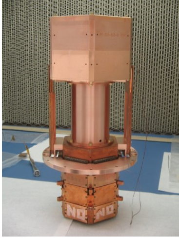
Figure 25: Left: Installation of a 100mm diameter crystal with the standard 75 mm CDMS readout hardware. Middle: Ionization energy spectra measured with G102a with four different electrodes. The 60-keV gamma peaks due to the ^{241}\text{Am} sources are clearly identified in the spectra. Right: Ionization collection efficiency as a function of bias voltage across the G102a crystal, measured using the positions of ^{241}\text{Am} 60-keV peaks.
