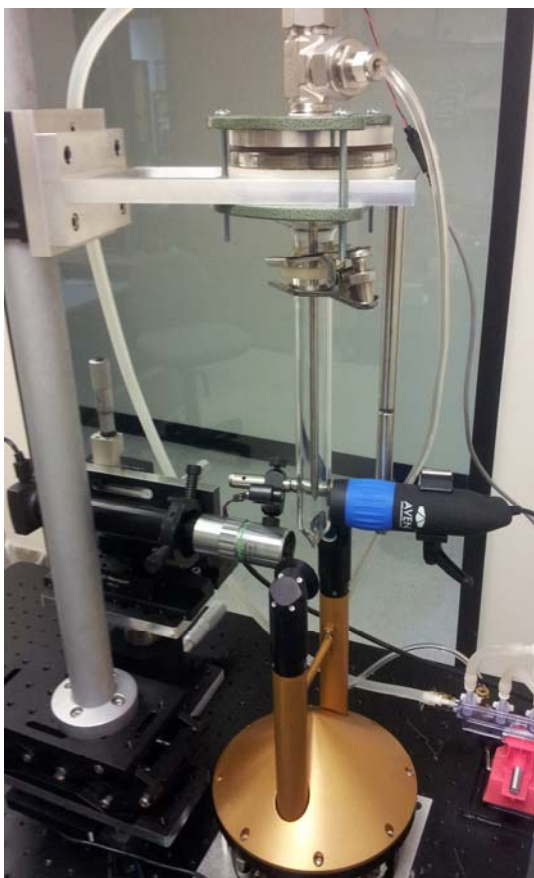
Figure 13: Calibration of a 2D-128 probe.
