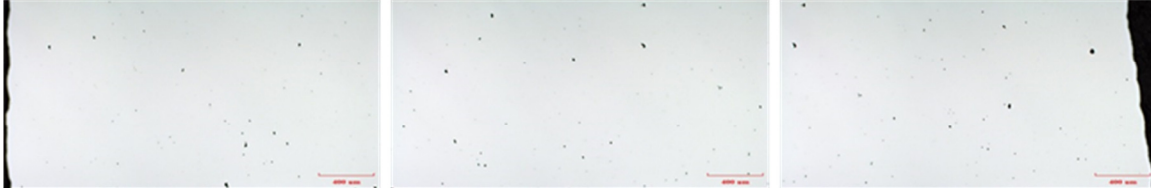
Figure 39. 316L SS Sample H2 micrograph of region ~1cm from necking, has irregularly shaped voids but not elongated
