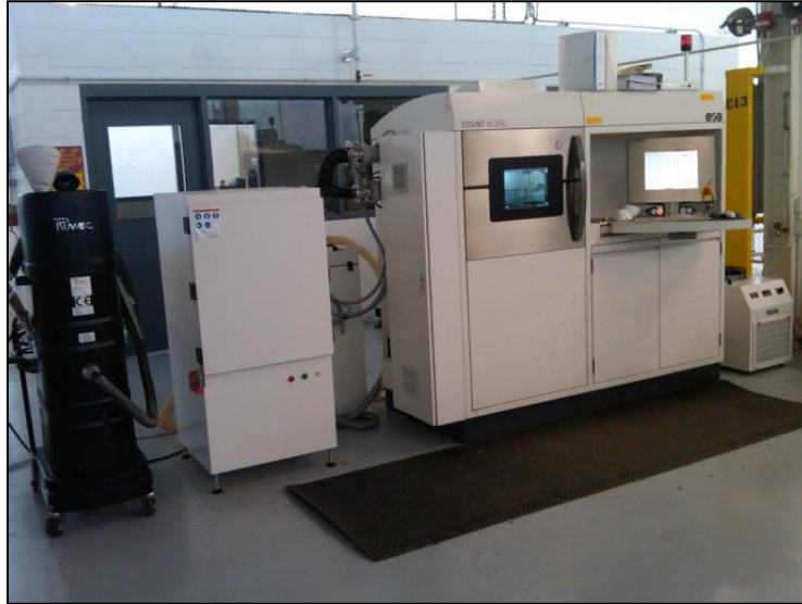
Figure 6. EOS M270 powder bed fusion system used to fabricate specimens in this study.
