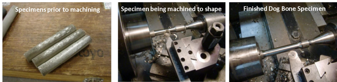
Figure 15. Machining of Inconel 600 samples to the standard test methods for tension testing of metallic materials—ASTM E8/E8M.
