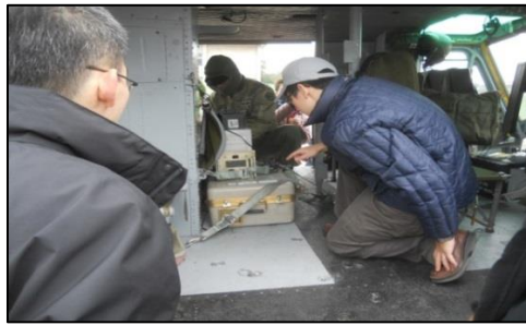
Figure 1. I-AMS SPARCS system installed in a helicopter and tested by radiation experts.
