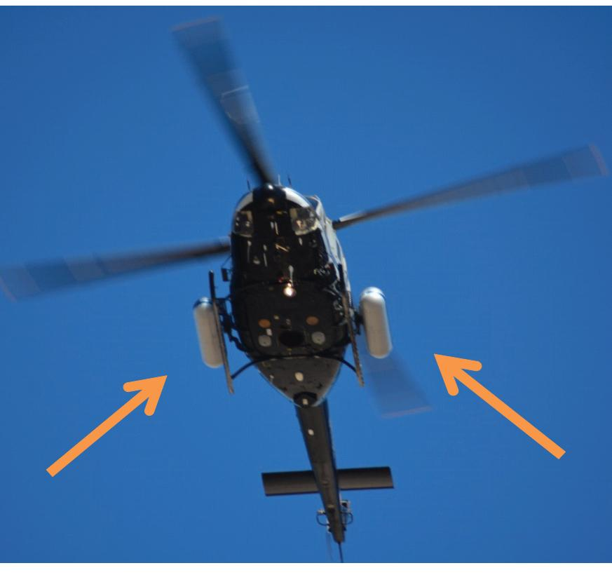
Figure 2: AMS Helicopter with gamma ray detectors attached
