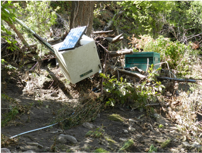
Figure 17 Damaged gage station in Water Canyon
