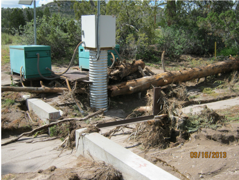
Figure 13 Debris at Sandia Canyon gage E125
