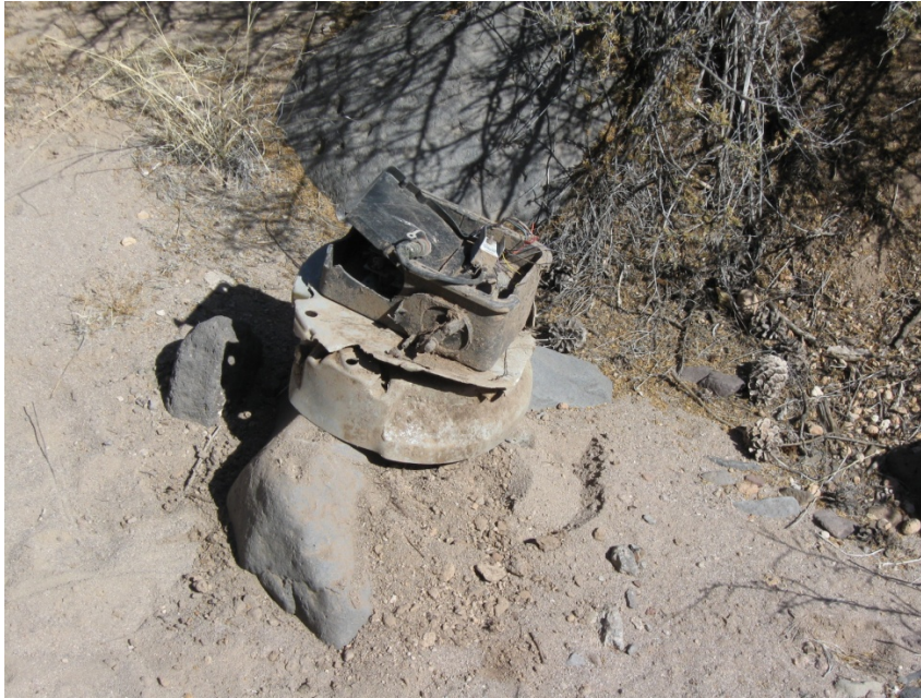
Figure 21 Damage to the top of an ISCO automated sampler
