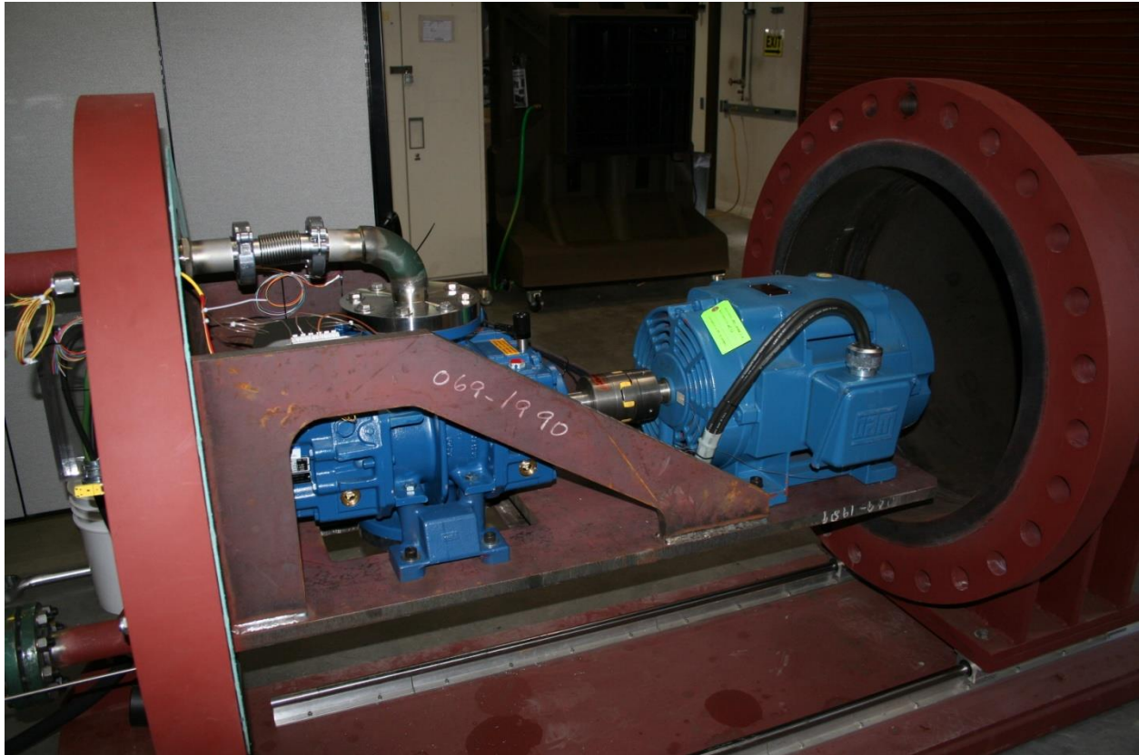
Figure 4. Close-up view of the blower, on the left, with motor. Motor is wired and blower exit piping is installed. (top left).
