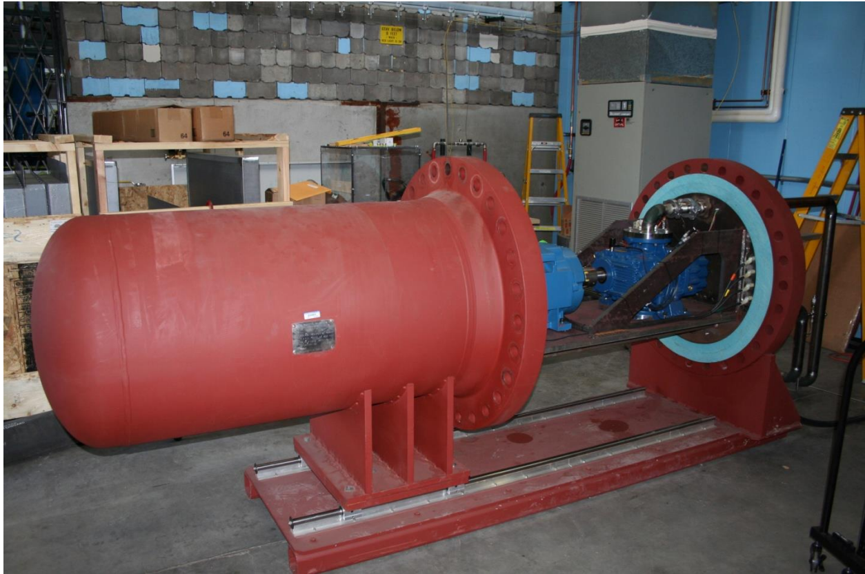
Figure 3. Vessel open, showing blower and motor.
