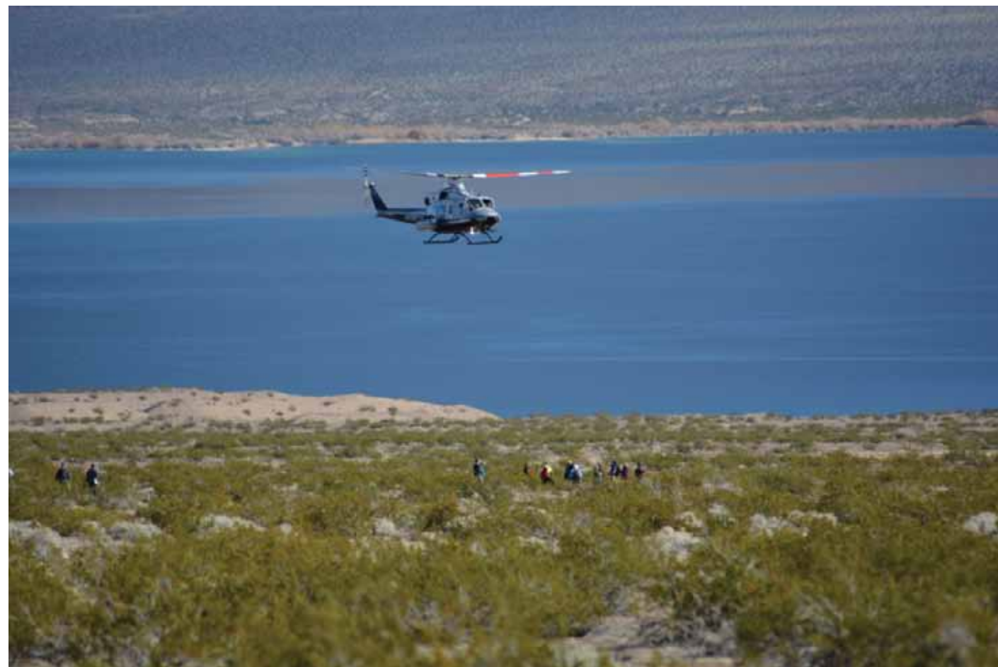
Figure 1: National Security Technologies, LLC. (NSTec) helicopter with sodium iodide (NaI) detector flying over the Lake Mohave field area
