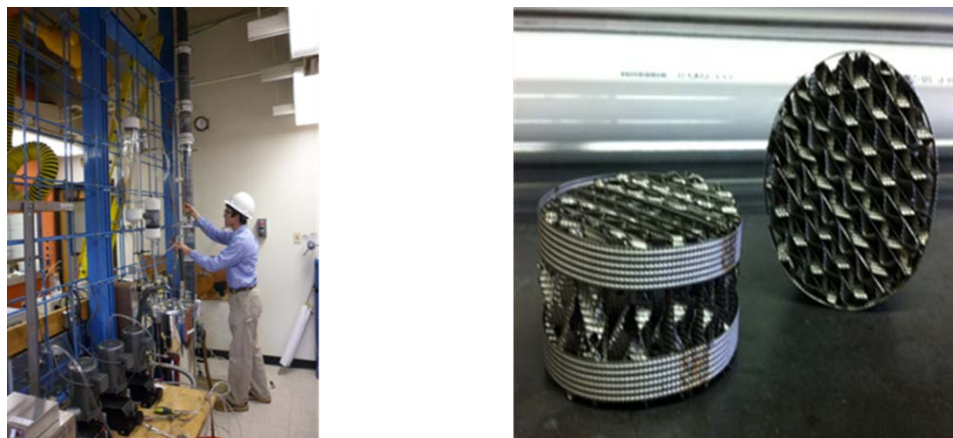
Figure 4.1. Adsorption Column and ancillary equipment (left); packing used in column (right)
