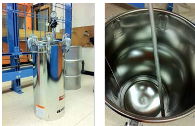
Figure 4.2. Stripper tank (left) and inside of tank with top removed (right)
