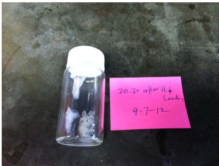
Figure 3.11. Photograph showing crystals recovered from the autoclave at the conclusion of the September 2012 VLE measurements for 20% PZ / 30% MDEA / 50% H 2 O (w/w) solvent. The crystals were observed when the solvent was removed from the autoclave at room temperature following the high CO 2 loading measurements.
