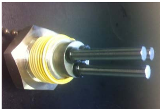
Figure 3.17. Metal coupons mounted for testing inside the chamber
