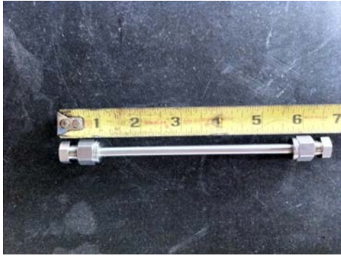
Figure 3.12. Sample holder for thermal evaluation (left), oven used in stability evaluations (right)
