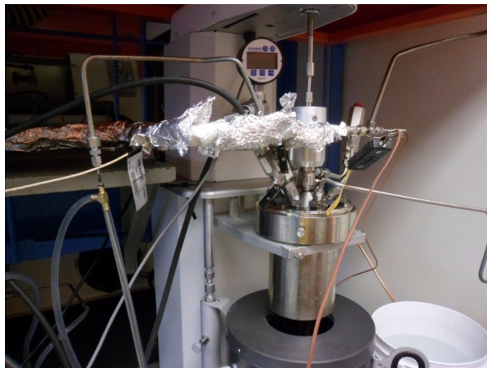
Figure 4.26. The autoclave system modified for the flasher tests
