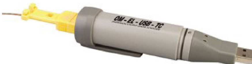
Figure 4-1. Thermocouple Data Logger used to Monitor Flue Gas Temperature in 10 houses
