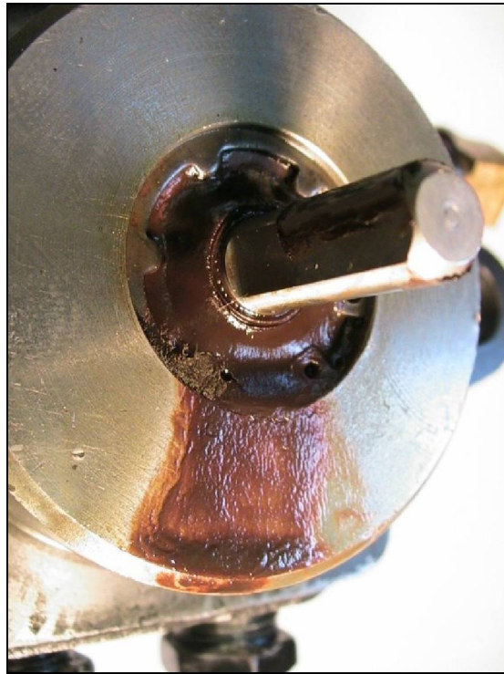
Figure 5-25. Oil pump with Viton seal failure
