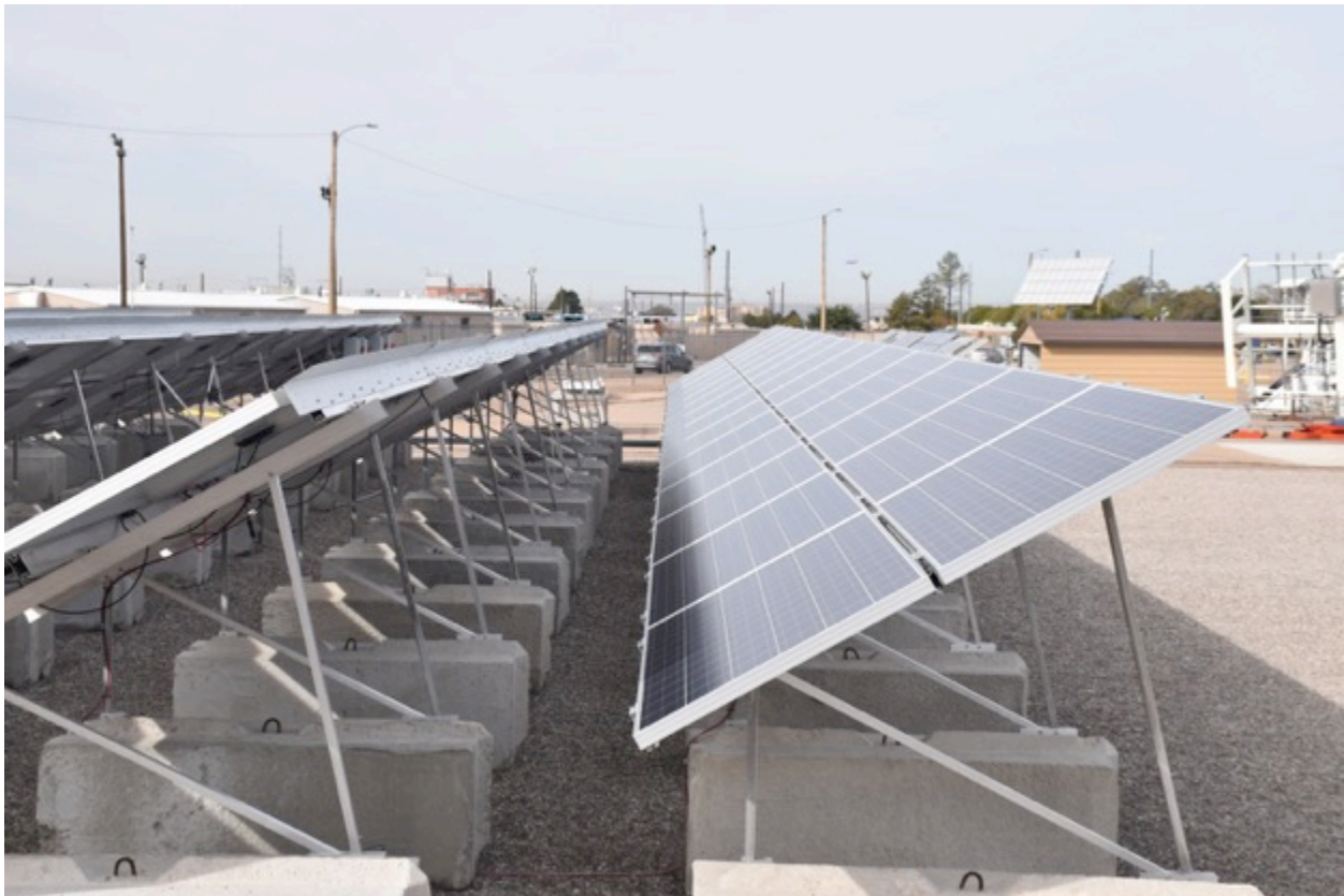
Figure 20. Testing of intentional row-to-row shading on the back row of Maxim's RTC array in New Mexico began in October 2015.
