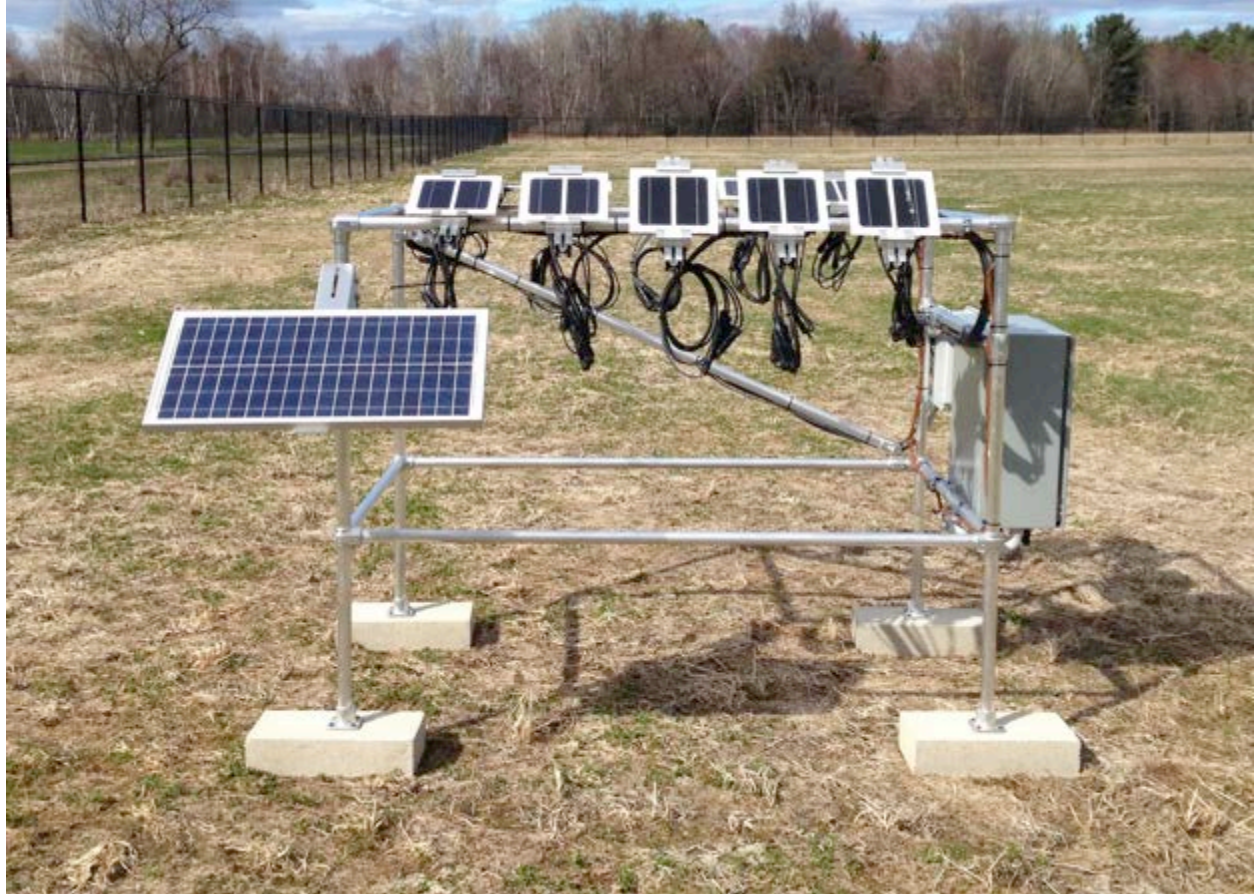
Figure 16. Soiling station at the VR RTC is measuring the effect of particulate accumulation on the energy output of split reference cells set at different tilt angles. The data logger ( grey box to the right ) is powered by the module mounted on the vertical post.
