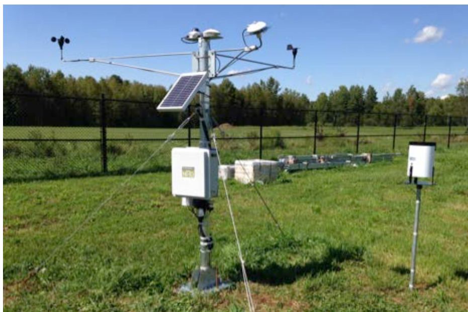
Figure 32. Solar resource assessment system installed at the Vermont RTC. The data logger (white box on tower) is powered by the solar module; irradiance and wind instruments are mounted at the top of the tower on booms; the rain gauge is to the right.
