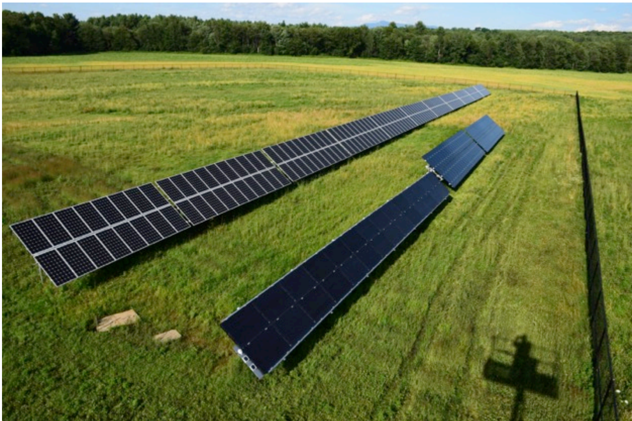
Figure 10. View of the PV arrays installed at the Vermont RTC as of the end of FY15. Array in back row is the 60-kW c-Si array. In the front row is the 6-kW baseline system in the foreground and the Stion systems in the background.
