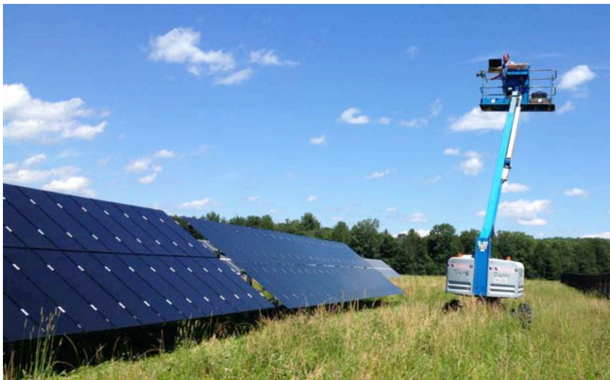
Figure 23. Sandia takes IR images of the Stion modules at the Vermont RTC.
