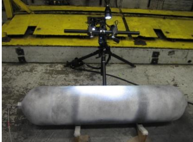
Figure 41. Vessel 13 measured with ARAMIS
