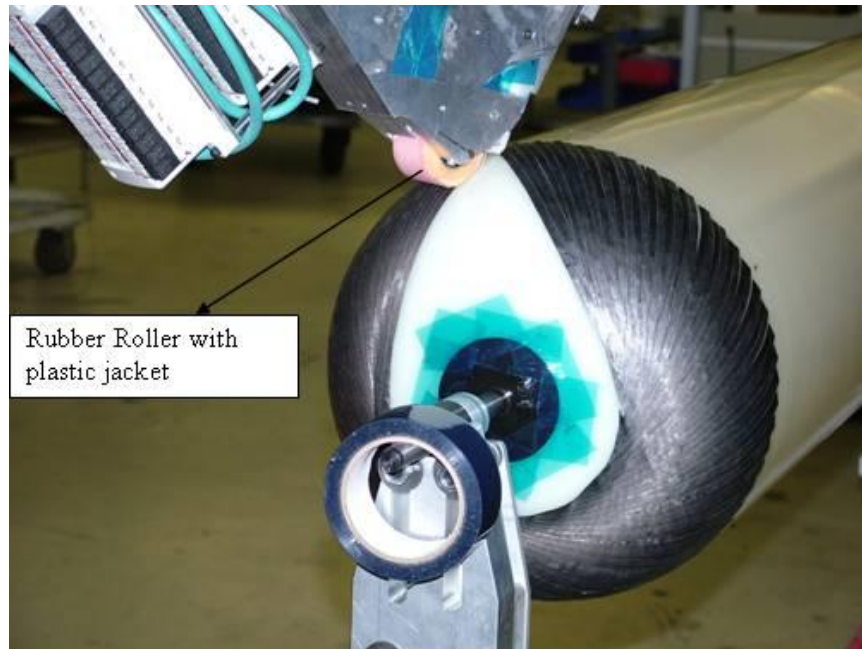
Figure 7. Material compaction from the rubber roller
