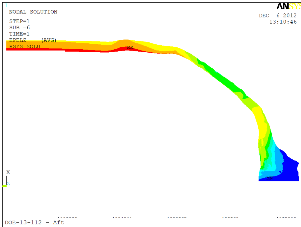
Figure 52. Aft end hoop strains on FEA without corrected dome buildup
