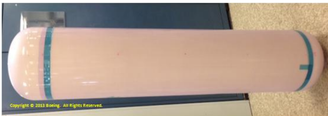
Figure 112. Completed process for stretching film onto liner
