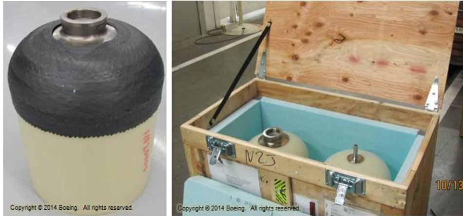
Figure 94. Forward cap new packaging (left), new reusable shipping container (right).
