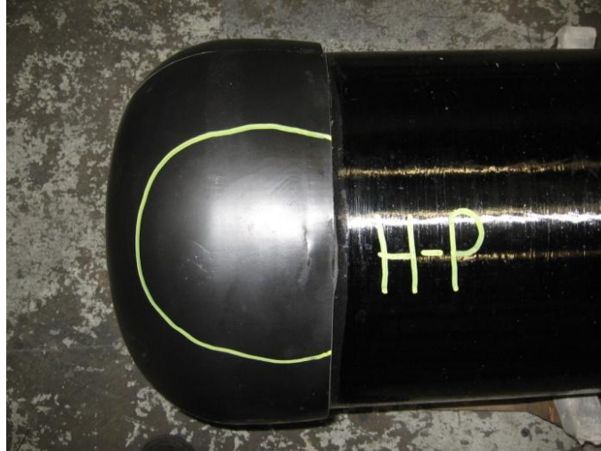
Figure 65. Foam dome deformation after impact
