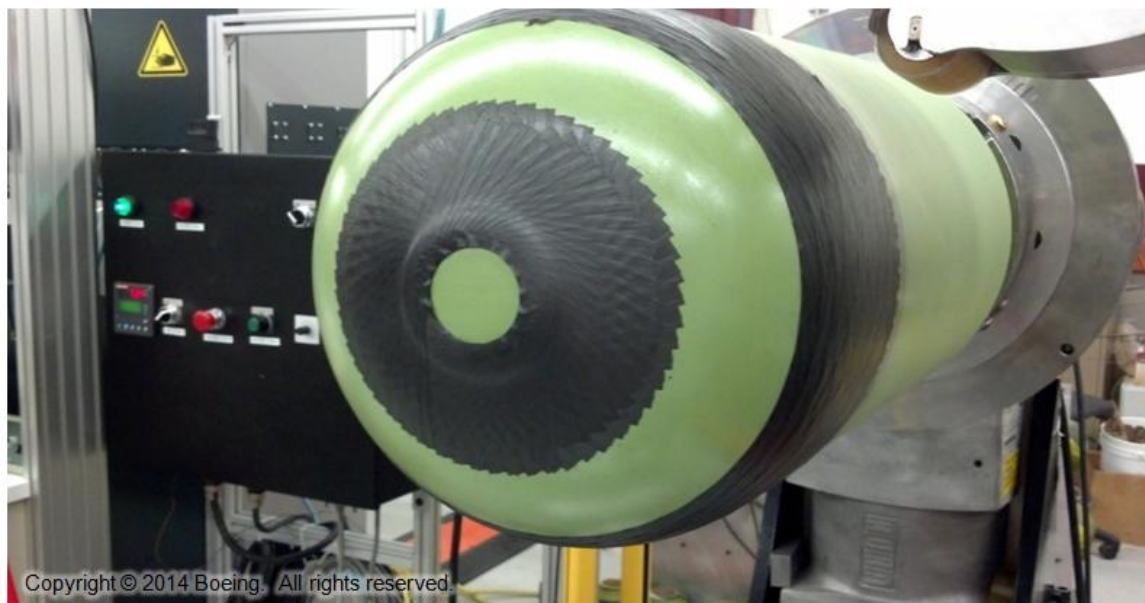
Figure 105. Layup of aft dome cap
