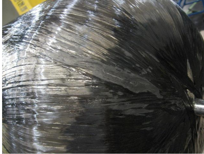
Figure 58. Ridge formed on the filament winding layer was filed away to avoid bridging for subsequent fiber layers
