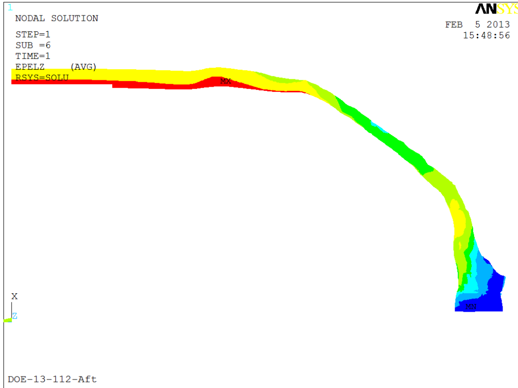
Figure 53. Aft end hoop strain on FEA with corrected dome buildup
