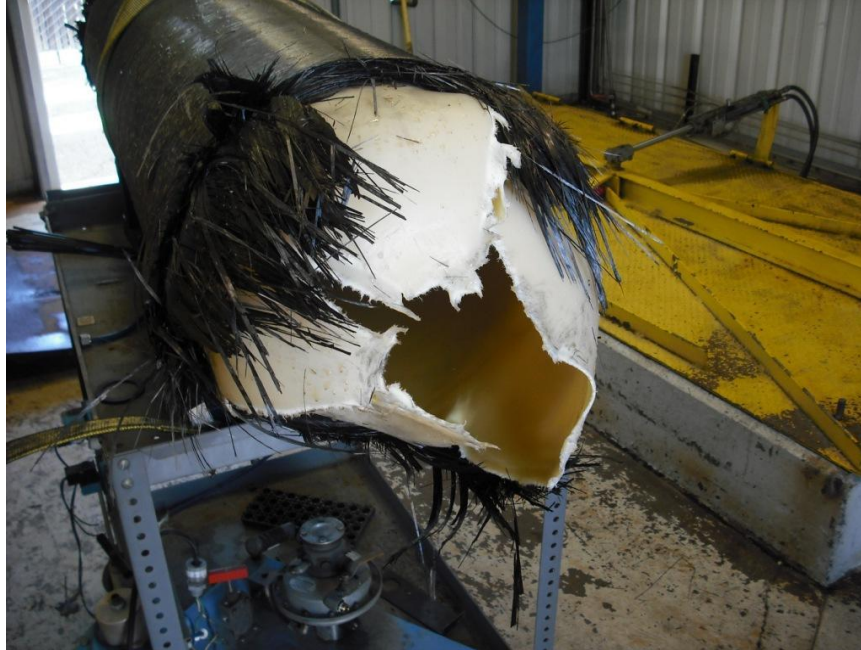
Figure 9. Vessel failure on the aft end
