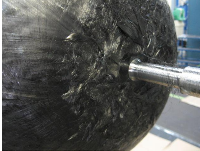
Figure 57. Chopped fiber was used to fill the dip between two end cap layers
