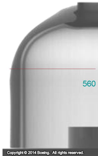
Figure 90. X-ray of the forward half-dome of Vessel 6
