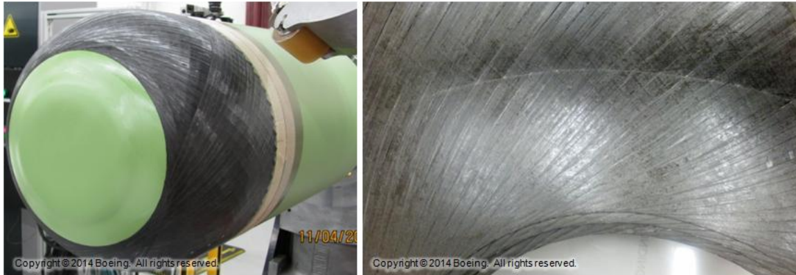
Figure 99. Picture showing the layup with minimal steering and two tows
