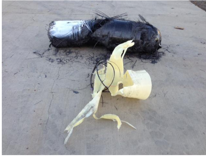
Figure 61. Vessel 16 burst mode was mid cylinder per design
