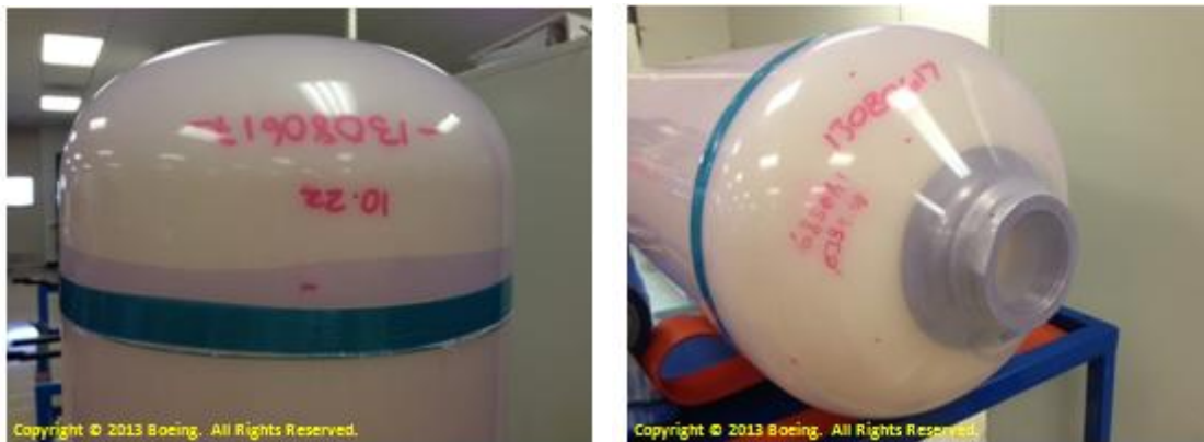
Figure 111. Picture of domes with stretch film by new method
