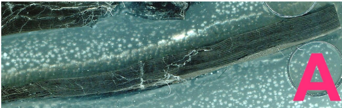
Figure 75. Photomicrograph of region “A” indicated in Figure 72. This particular region is from the second layer of tow-placed material extracted from the damaged area of the dome. Some fiber waviness is apparent.
