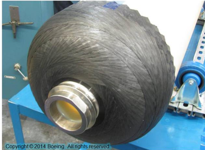
Figure 85. Forward end fit of AFP end cap on liner with thermoformed shear protector
