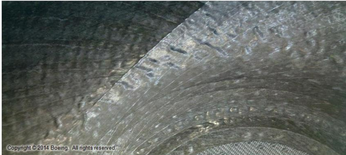
Figure 95. Picture showing wrinkles in layup of Vessel 9
