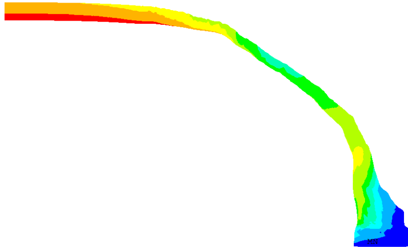
Figure 25. Hoop strain contour plot of Vessel 13 aft end
