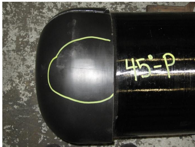
Figure 66. Foam dome cracked after impact
