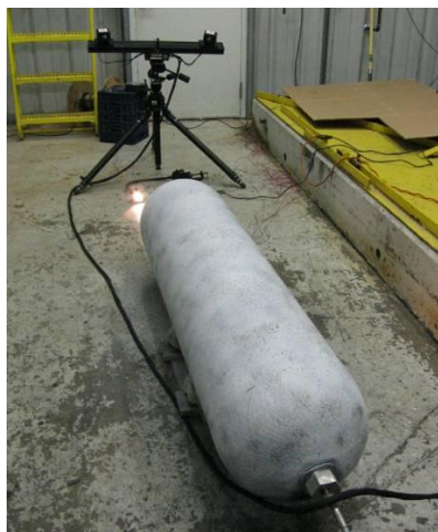
Figure 12. ARAMIS measures the displacement of dots on vessels and evaluates the strains
