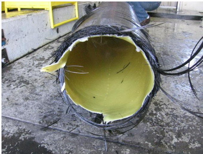
Figure 15. The aft end cap failed at edge of AFP layers
