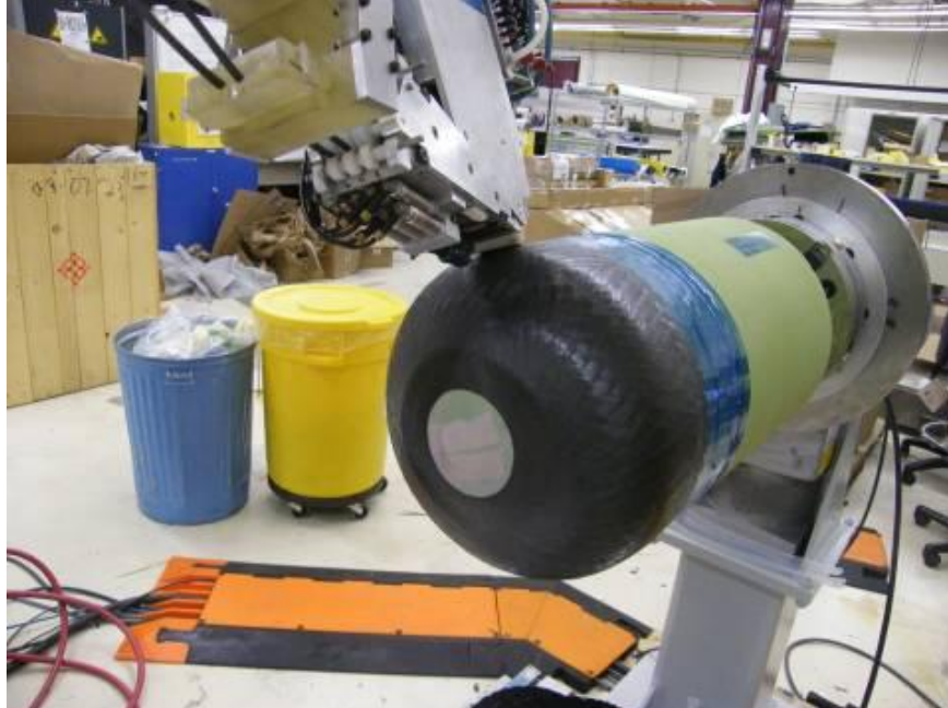
Figure 8. Semi-rigid foam tooling
