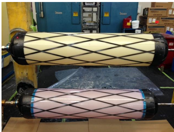
Figure 60. Released film installed for the bottom vessel planned for cycle test
