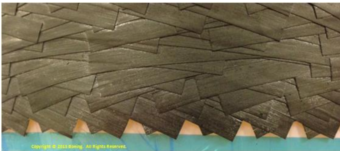
Figure 108. Placement of dome cap on liner
