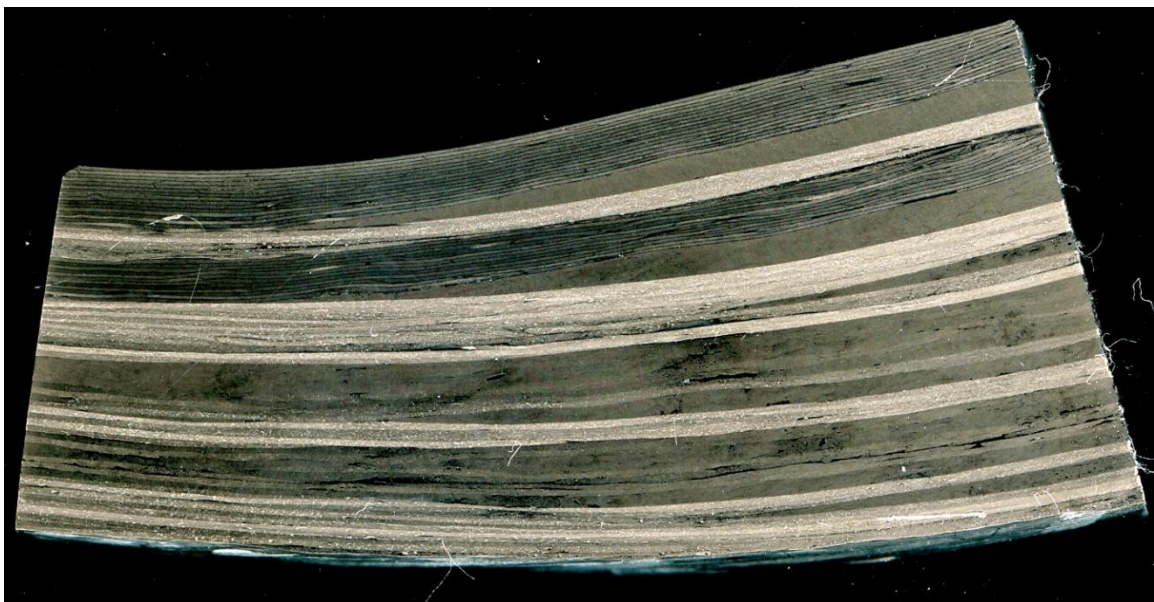
Figure 73. CT scan of Vessel 3 forward end
