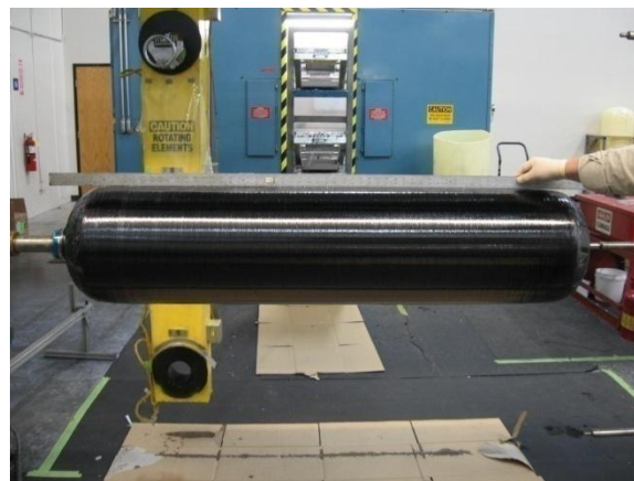
Figure 34. Hoop layers relocated to eliminate gap
