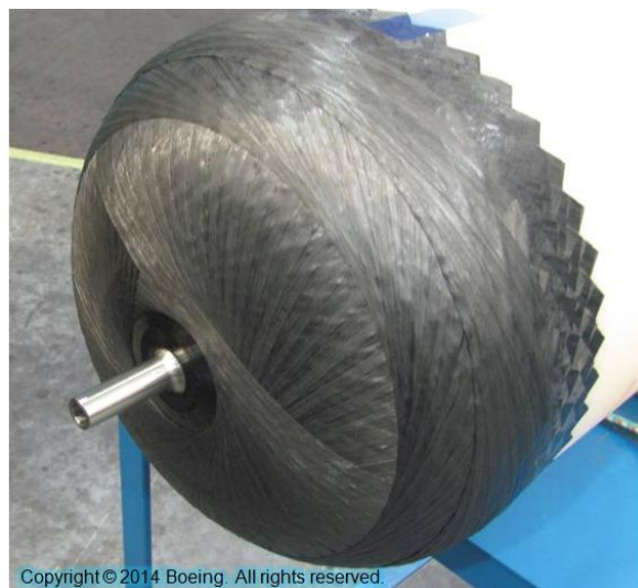
Figure 87. Aft end fit of AFP end cap on liner with thermoformed shear protector
