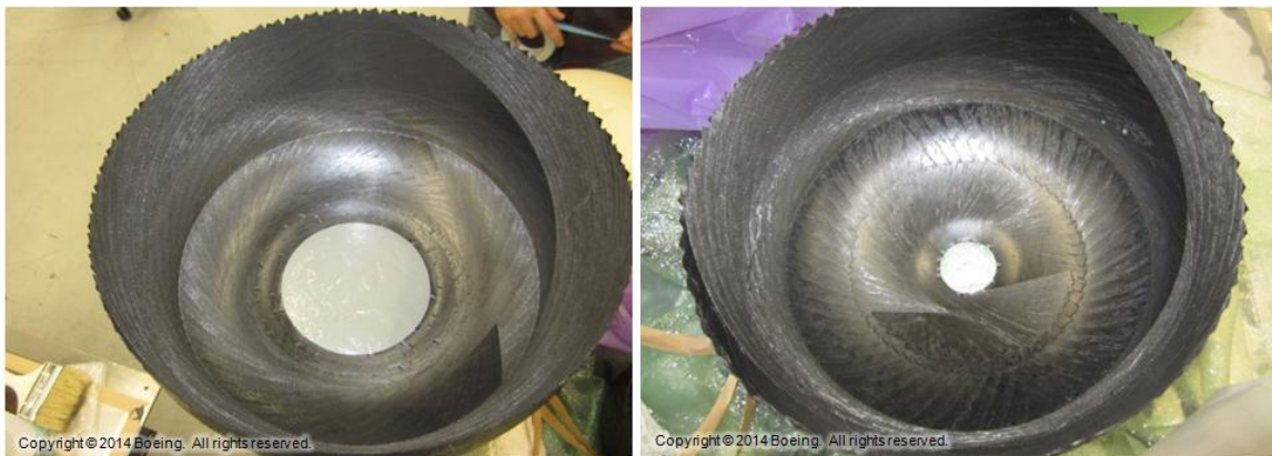
Figure 107. Pictures of forward and aft end cap internal surfaces (after vacuum bagged)
