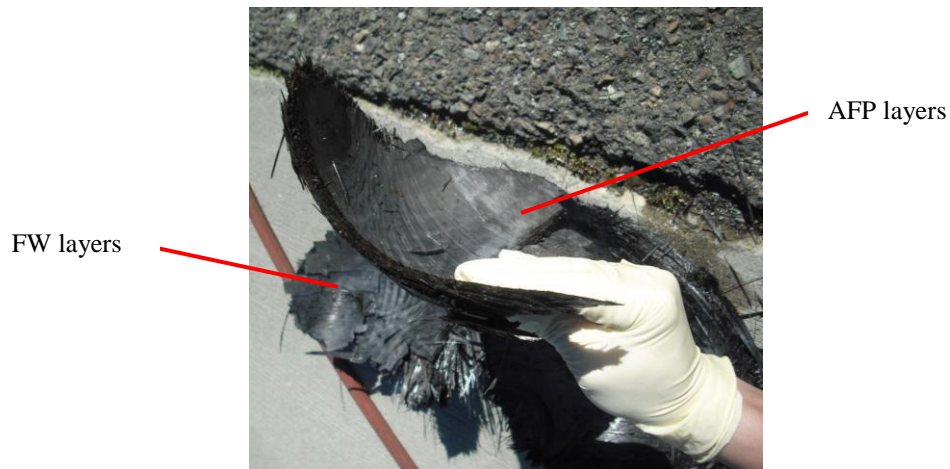
Figure 10. Composites from the aft end showing dryness between FW and AFP layers
