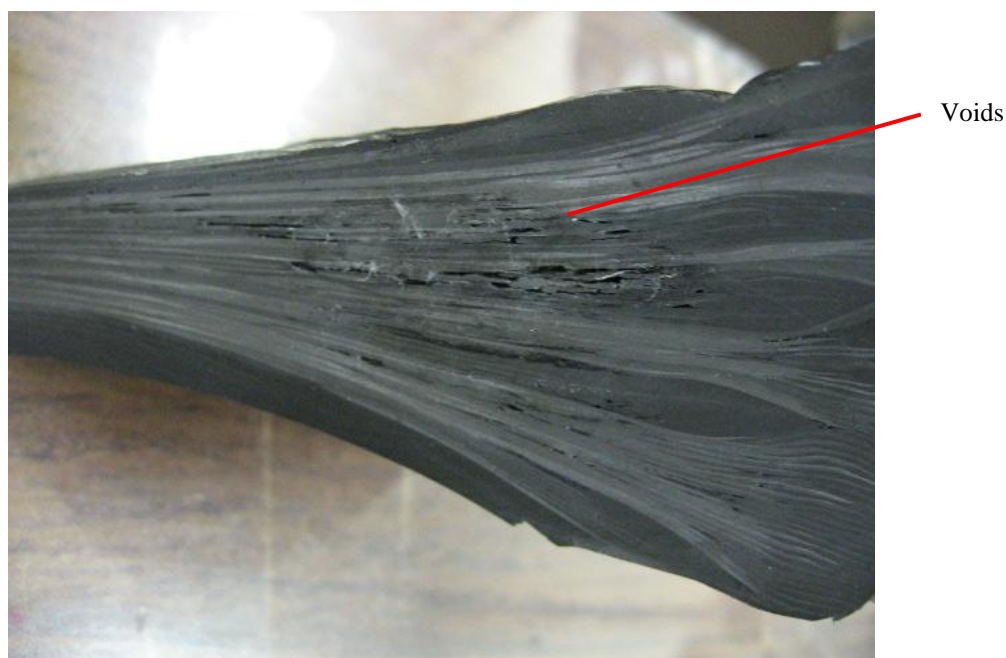
Figure 11. Voids shown in the sectioned aft dome
