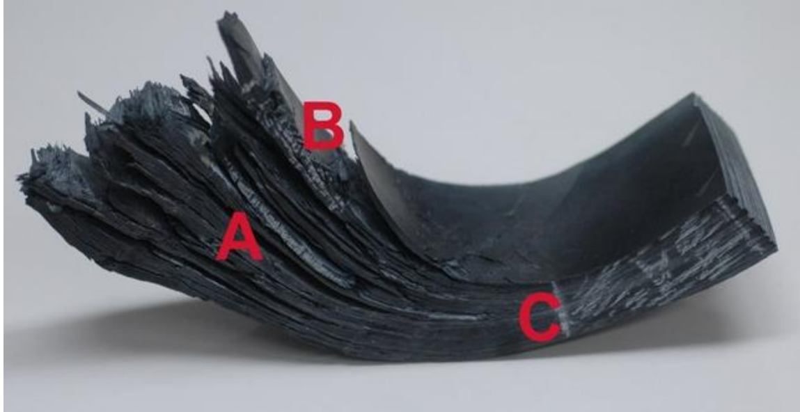
Figure 72. Section cut from the forward dome region of Vessel 3
