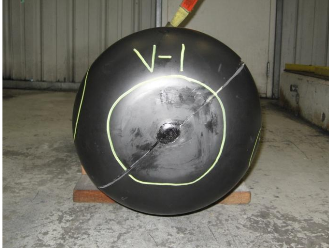
Figure 64. The foam dome was cut to remove material to fit onto composite dome
