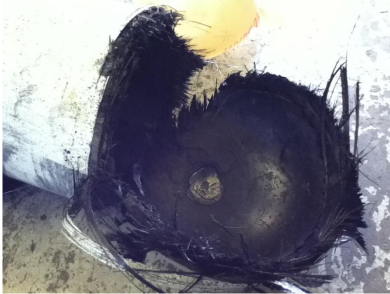
Figure 23. Vessel 7 aft dome after burst test
