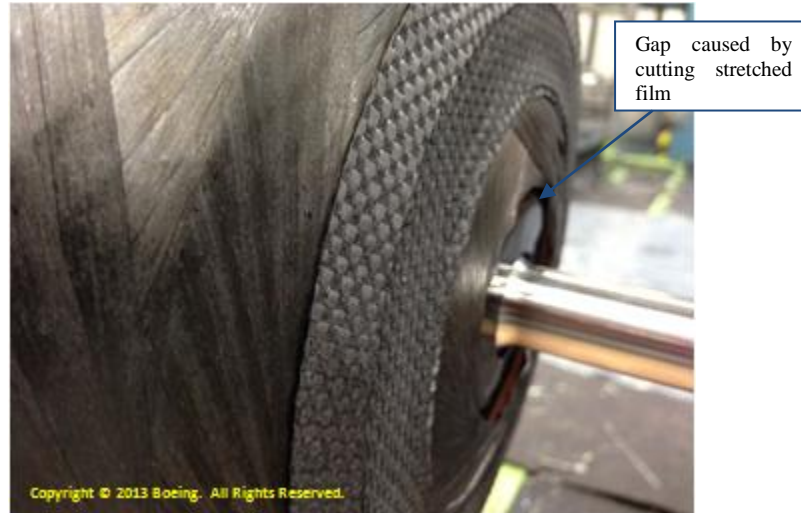
Figure 110. Picture of gap caused by cutting stretched film
