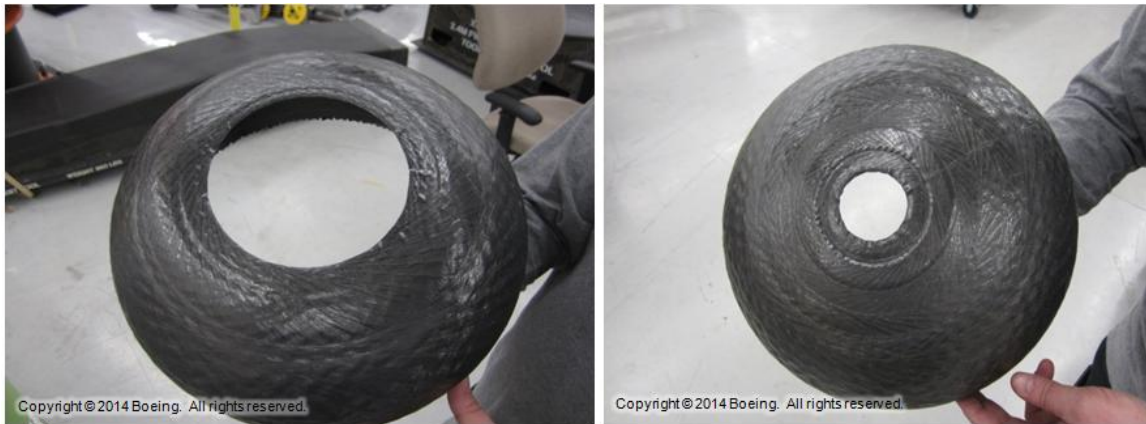
Figure 106. Pictures of forward and aft end caps external surfaces (after vacuum bagged)
