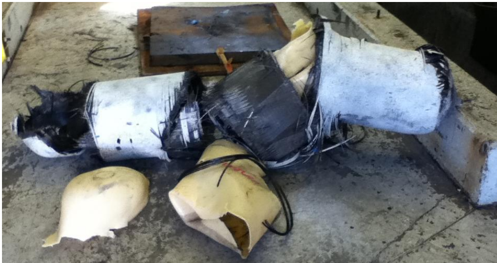
Figure 14. Vessel 7 ruptured in mid cylinder, as predicted by the model.
