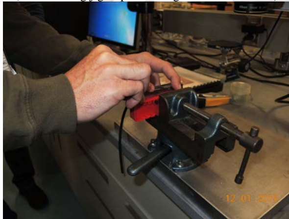
Photo 5 (Vice holding jig in place using razor blade to cut)
