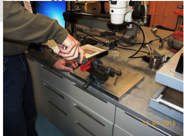
Photo 6 (Vice holding jig in place using utility knife to cut)
