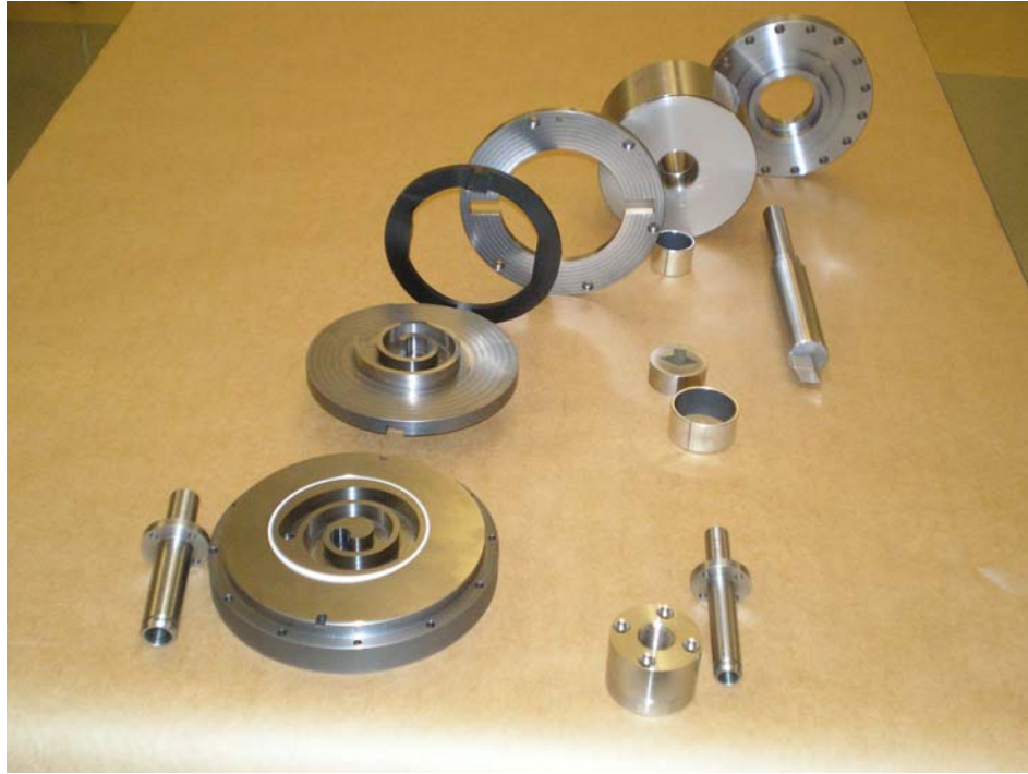
Figure 4-1: Fabricated Parts of the Scroll Expander
