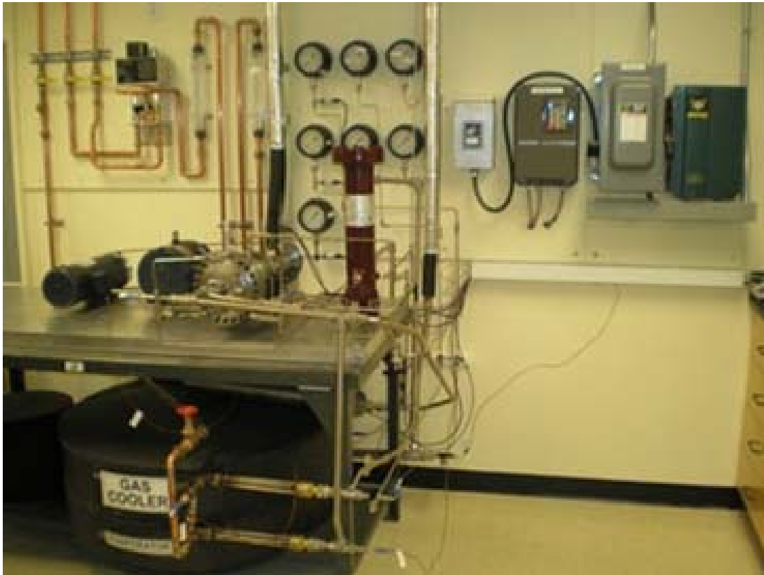
Figure 5-10: Completed Test Loop
