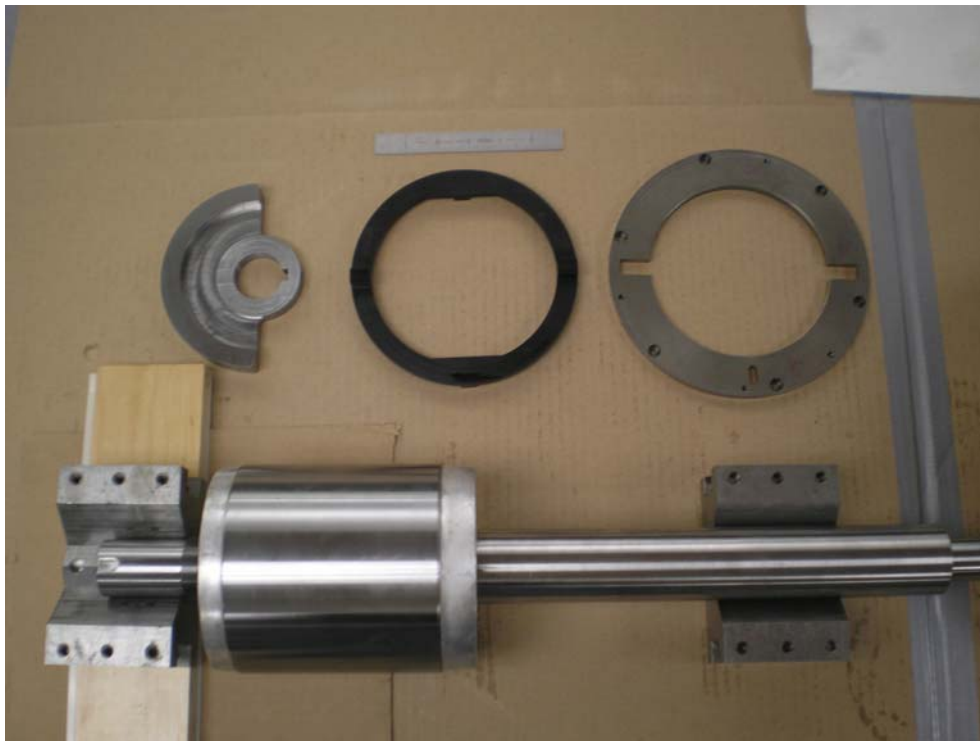
Figure 7-5: Compressor Moving Parts (Shaft, Motor Rotor, Oldham Coupling and Counterweight)
