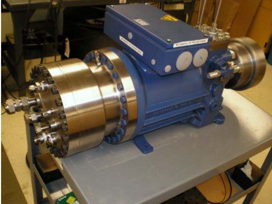
Figure 7-6: Compressor and Expander Housings Assembled with Bock Compressor Housing
