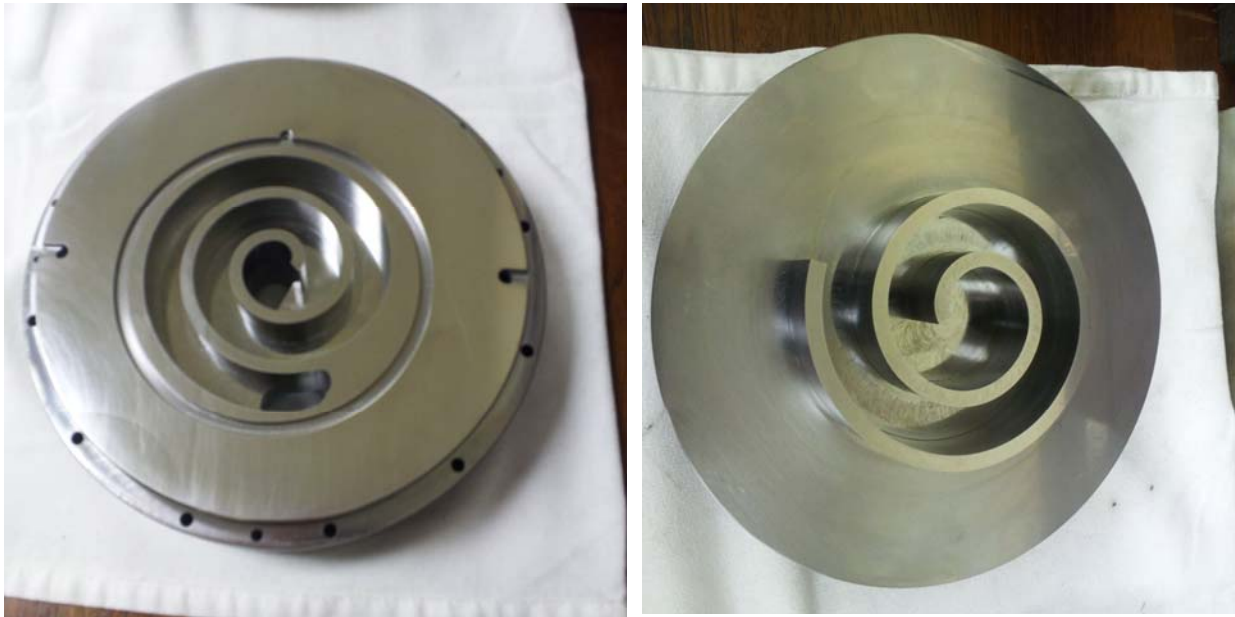
Figure 7-1: Fixed and Orbiting Scroll Parts for the Compressor
