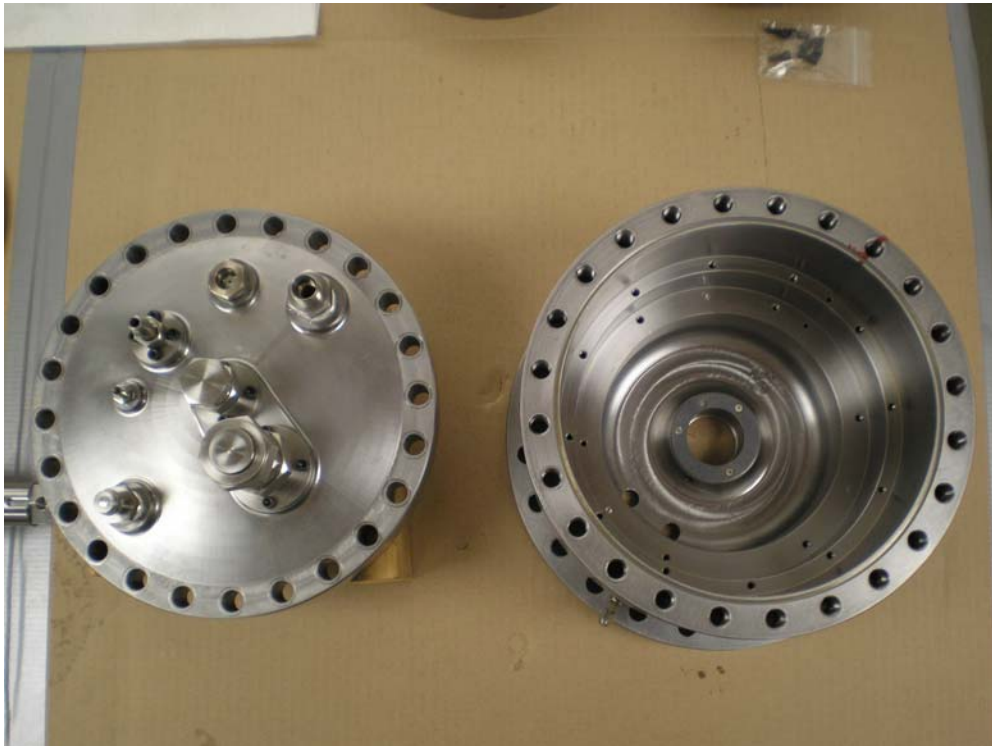
Figure 7-2: Bock Compressor Housing with Motor Stator
