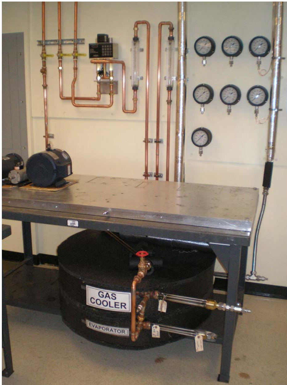
Figure 5-5: CO 2 Gas Cooler and Evaporator in the Test Loop with CO 2 Piping
