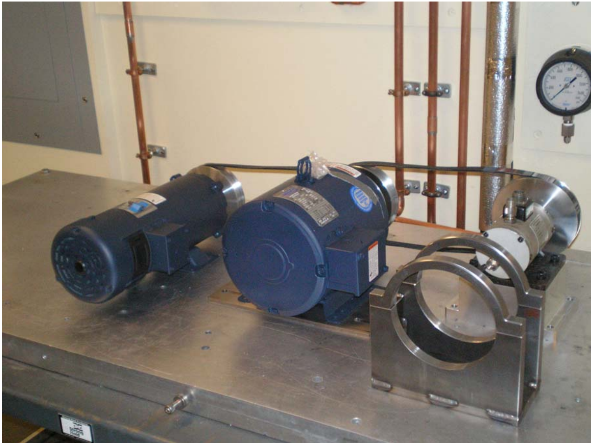
Figure 5-8: Motor and Generator Placed on Mounting Plate
