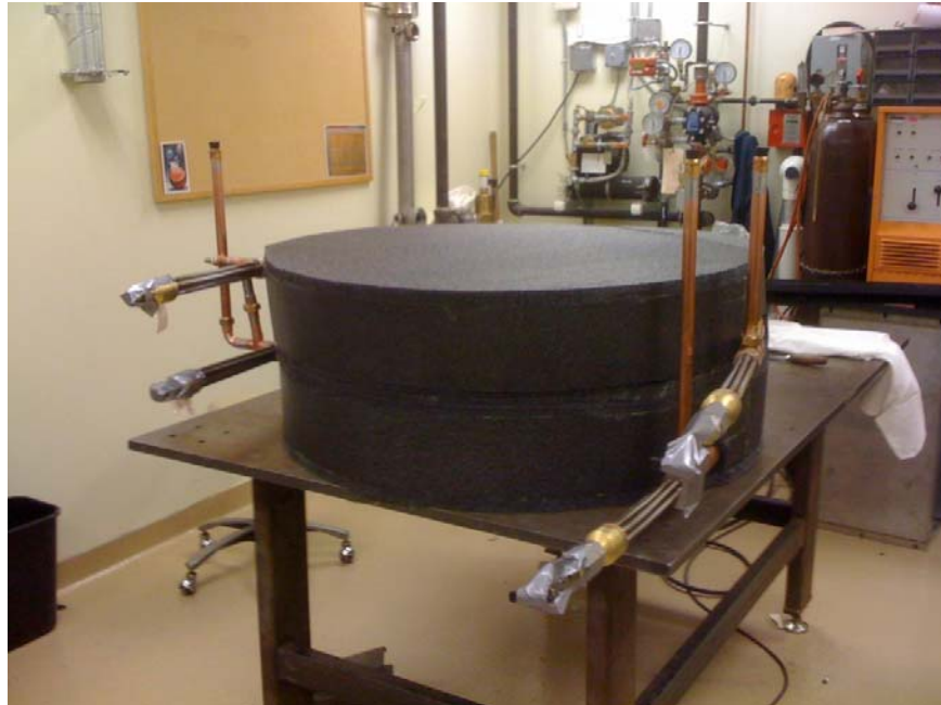
Figure 5-4: Completed CO 2 Gas Cooler and Evaporator (the Gas Cooler is on Top of the Evaporator)
