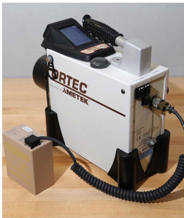
Figure 15: Transpec-100, rear view showing the PDA
