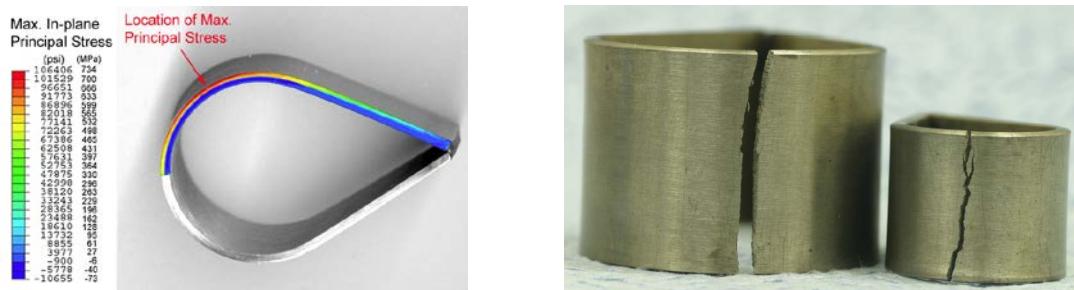
Figure 43(a). Location of stresses in a teardrop calculated using finite-element analysis. 43(b). 304L teardrops after exposure to boiling magnesium chloride solution.
