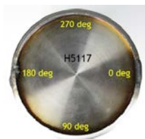
Figure 29. Photograph of Lid of 3013 inner container H5117 showing two large weld defects.
