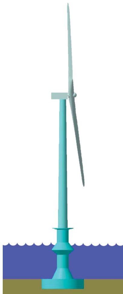
Figure 7.5. Gravity base foundation.
