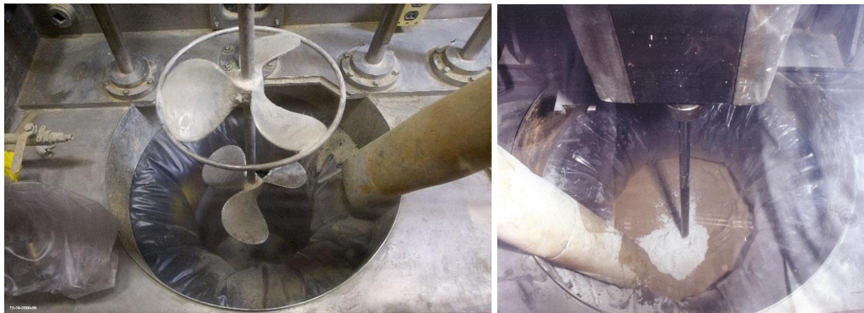
Figure 5 Cementation glovebox operation at TA-55
