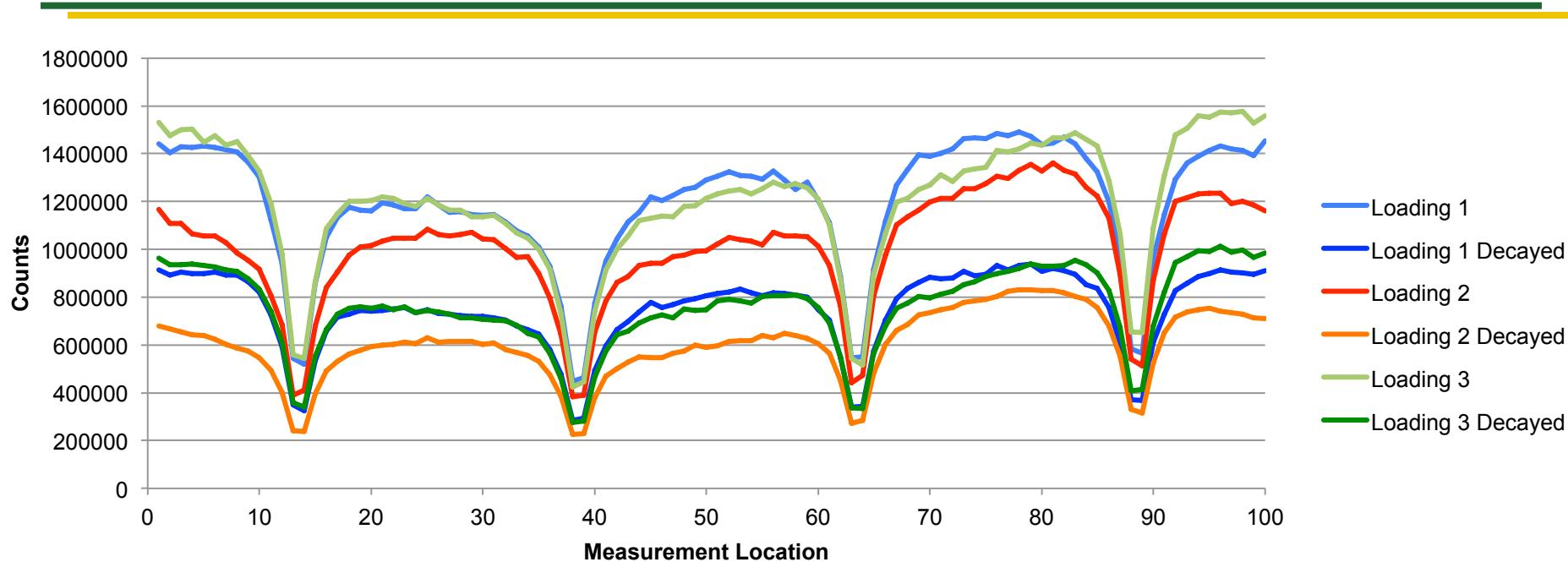
20 years worth of decay dramatically lowers the count rates, so the normalization is needed for comparison of profiles, but count rates can be indicative of missing assemblies if assembly source strength can be estimated reliably over time.
