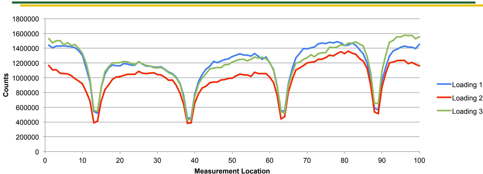
Loading 2 produces significantly lower measurements. Lower measurements expected due to older fuel, with lower neutron emission rates.
