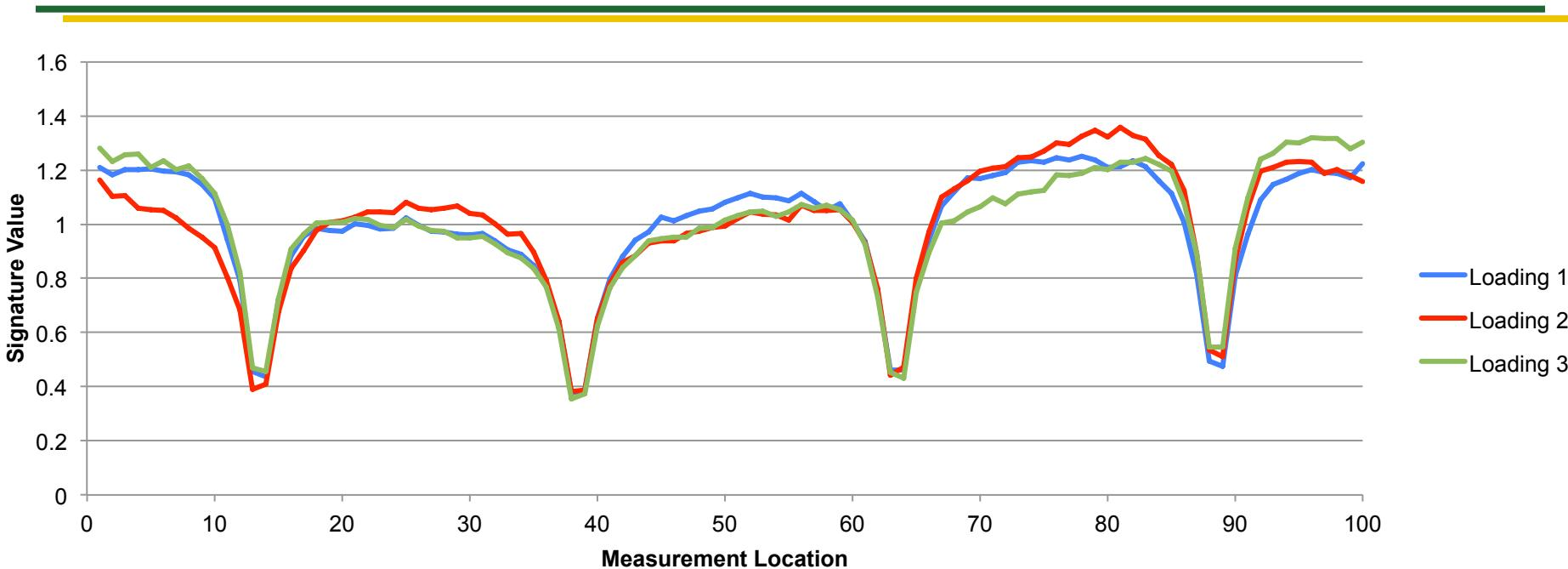
Visible differences in the profile are evident. If more than 5 SV are greater than 5% different in comparison to another measurement, no match.
