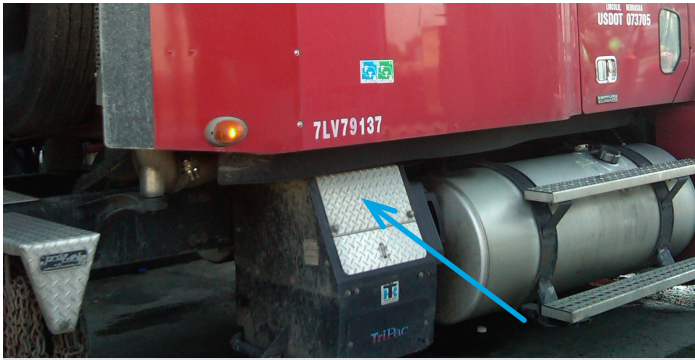
A truck equipped with an APU. APUs provide power for climate control and electrical devices. Photo courtesy of Terry Levinson.
