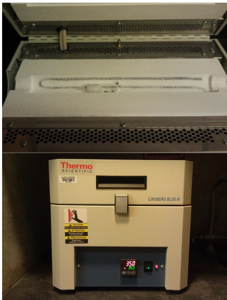
Figure 3.6 Top: individual crystals that have been picked from a growth and resealed in evacuated silica tubes for annealing. Bottom: annealing furnace stabilized at 350°C.
