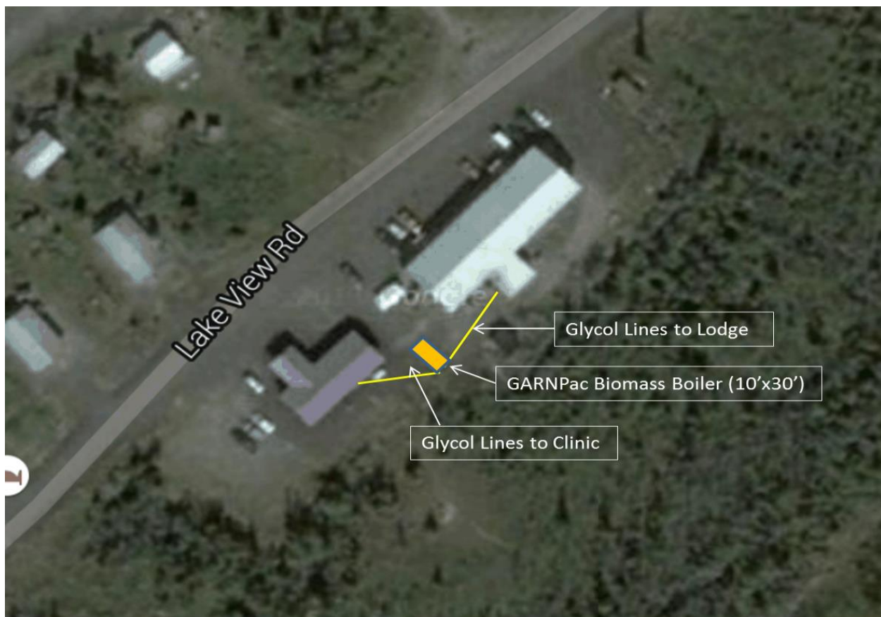
Figure 5. Aerial view of the Minto Lakeview Lodge (Right) and Minto Clinic (Left) and the approximate location of the biomass boiler slated for construction summer 2016 which will heat both buildings with locally sourced cord wood
