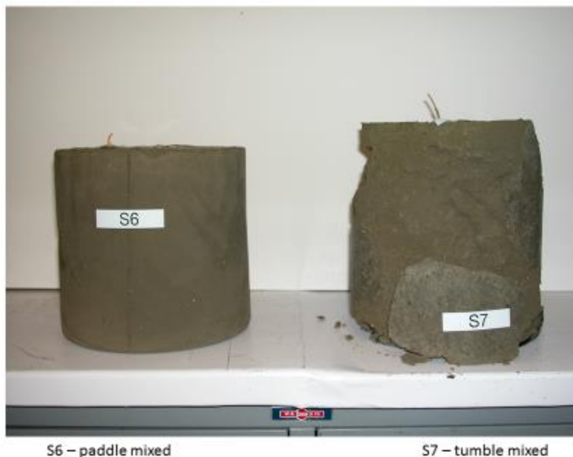
Figure 4 Comparison of cement made with agitation and via rolling “tumble”
