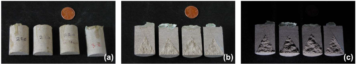
Figure 3.1: Images of short-rod fracture samples, (a) outside view, (b) inside fracture surface has propagated completely, and (c) inside fracture surface with an angled illumination to capture detailed crack features Rinehart et al. [14]
