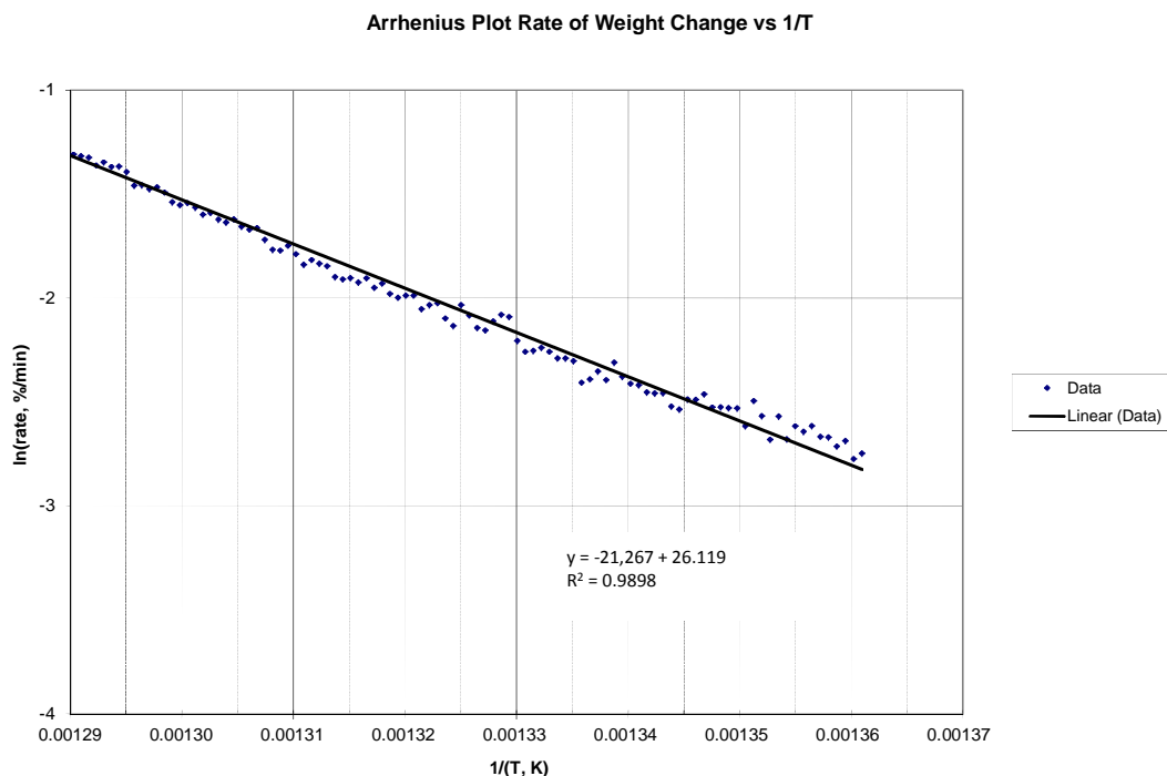
Figure 43. Arrhenius plot of rate of weight change vs temperature for the VK115D on fiber.
