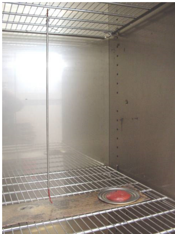
Figure 88: Tube and saucer sample in the oven at 150°
