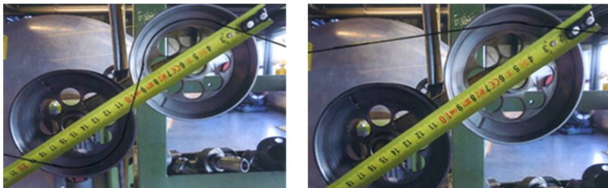
Figure 134: Fiber along the pay-off rolls before (S-shape) and after the broken fiber.
