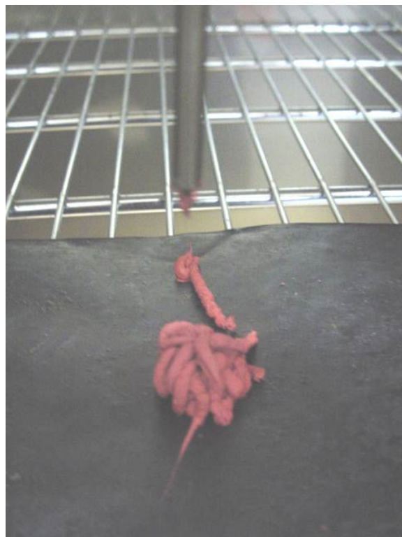
Figure 89: Silicone pushed out the tube at 200°C
