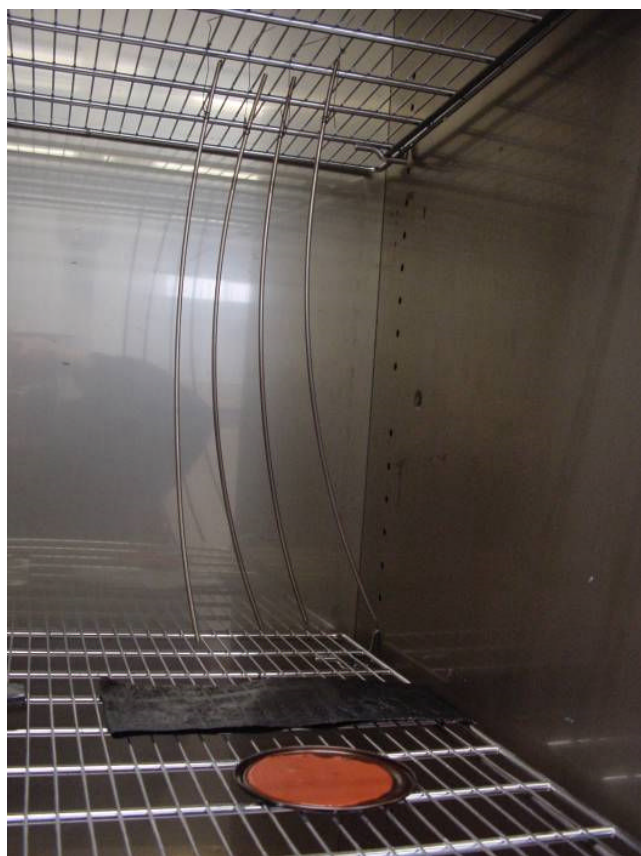
Figure 94: Tubes and a saucer filled with Loctite JS533 in an oven at 300°C.
