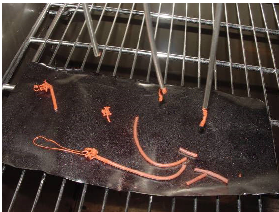
Figure 93: More silicone pushed out the tube at 300°C
