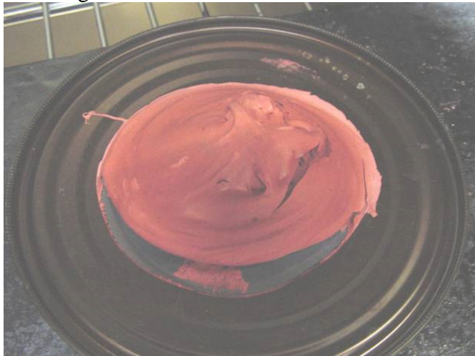
Figure 86: Loctite 5612 at 300°C
