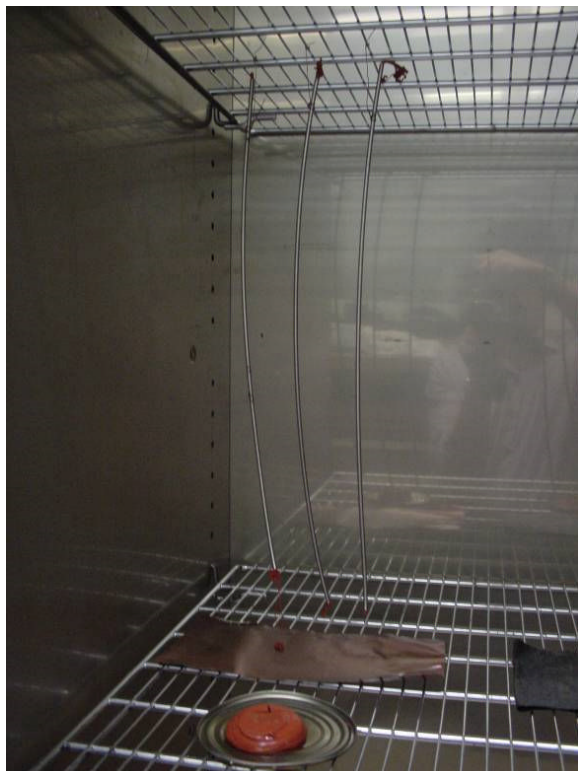
Figure 90: Tube and saucer sample in the oven at 150°.
