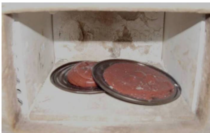
Figure 97: Loctite 5399 and JS533 in a small oven at 350°C
