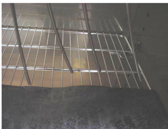
Figure 95: Tube filled with JS533; nothing is pushed out at 300°C.
