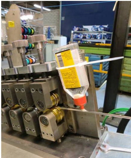
Figure 105: Lubrication of the steel strip
