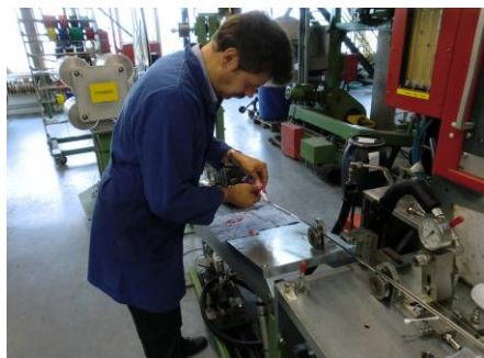
Figure 107: Manual injection of the plug
