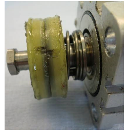
Figure 122: The spring inside the pneumatic cylinder is pressed at injection and it sprung back subsequently
