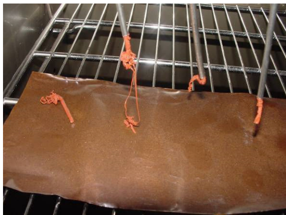
Figure 92: Silicone pushed out the tube at 250°C
