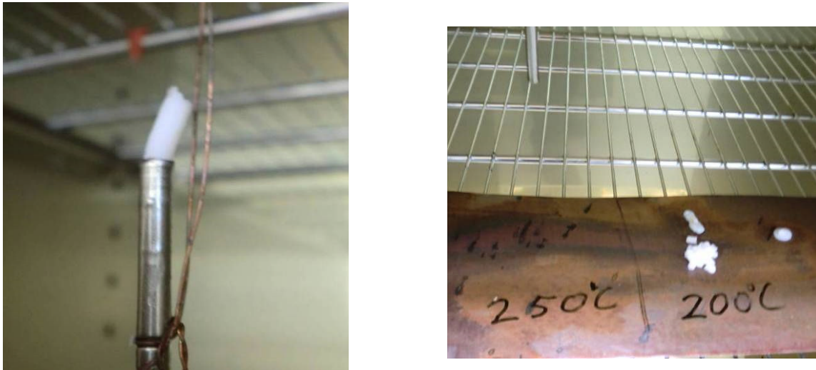
Figure 103: HT192 is pushed out of the metal tube, top and bottom
