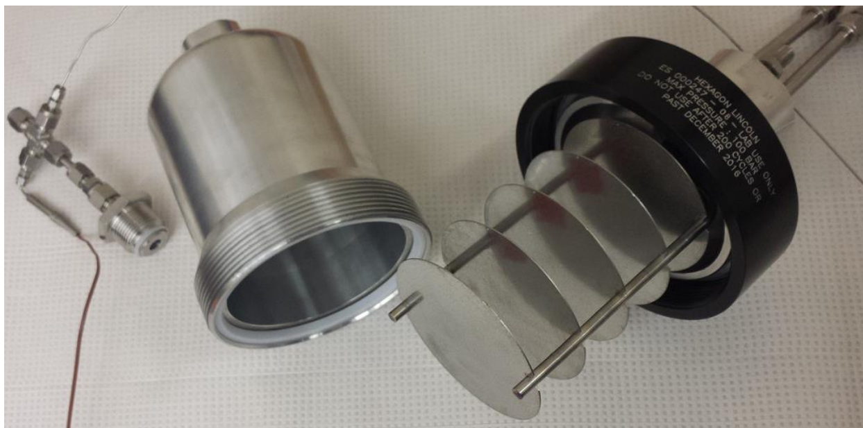
Figure 54: Five plate MATI installed in the large plug and smaller dome of the collared pressure vessel for initial system debugging.
