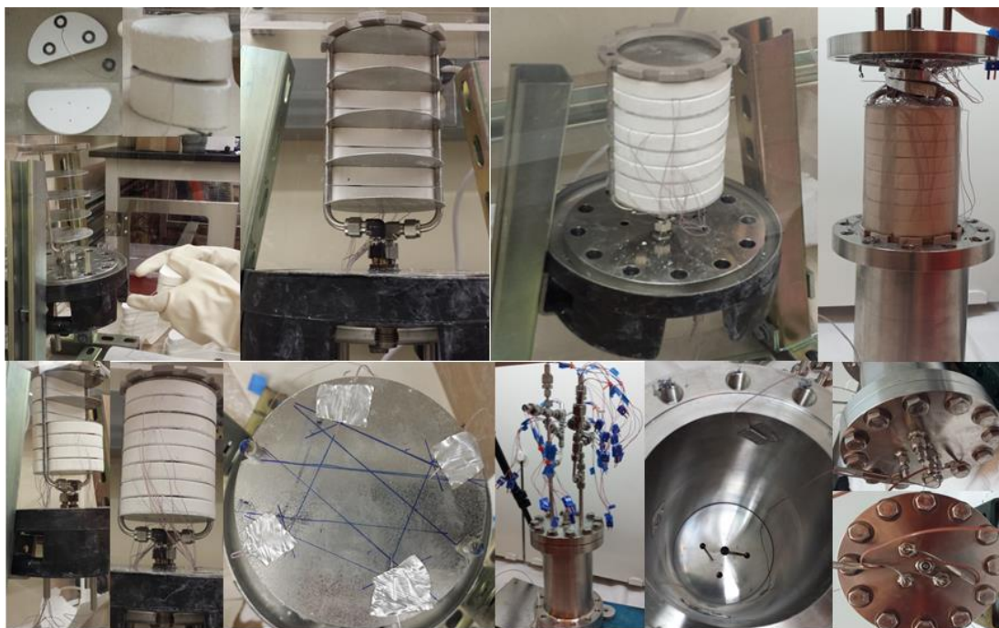
Figure 55: Various steps of assembly process and fully assembled flanged pressure vessel.
