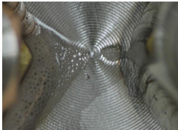
Figure 40.: Pinhole leak on flange
