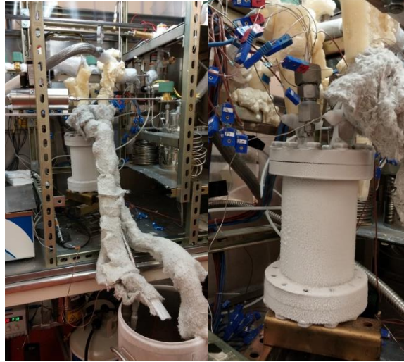
Figure 60: MATI during adsorption with subcooled LN 2 and precooled N 2 at 25 bars
