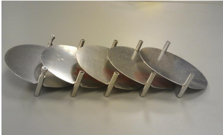
Figure 45: Individually brazed MATI cooling plates
