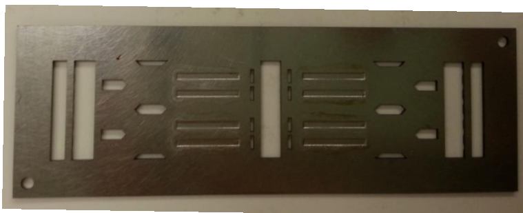
Figure 20. Etched channels on the back side of a channel.
