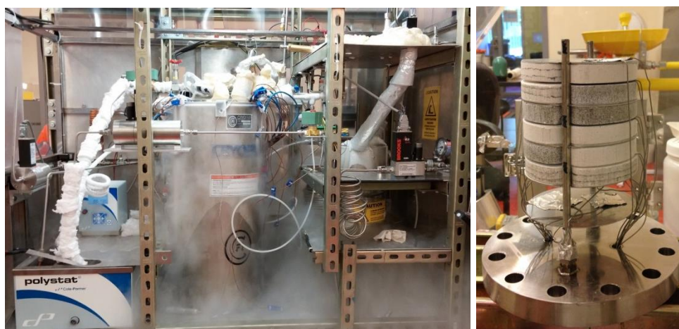
Figure 63: Experiment apparatus during submerged adsorption test (left); MATI with improved thermocouple placement and bed re-location (right)
