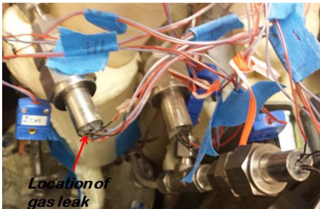
Figure 56: Custom made thermocouple pass-through that demonstrated leaks at wire upon the addition of \text{LN}_2 to research Dewar containing pressure vessel.
