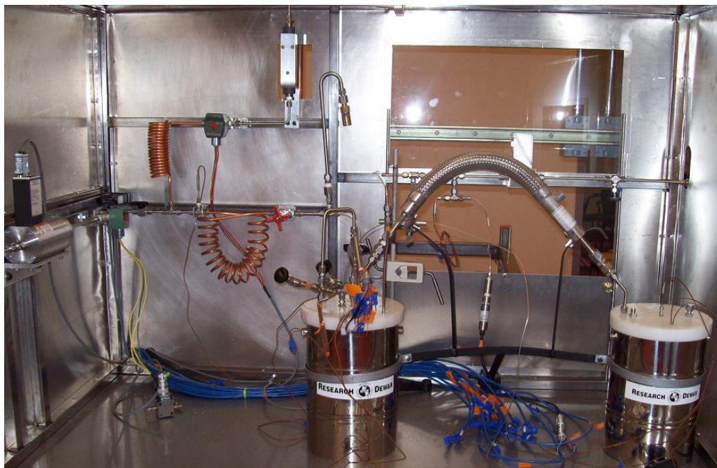
Figure 35: Fully assembled integrated testing system inside of sheet metal enclosure.
