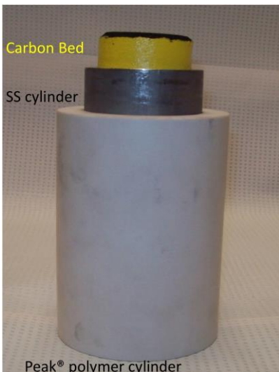
Figure 49.: Exploded view of the Carbon Bed placed into SS cylinder and PTFE cylinder.
