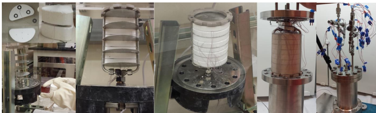
Figure 51: 1 st MATI assembly process
