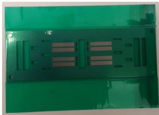
Figure 19. A combustor shim covered with mask for etching.
