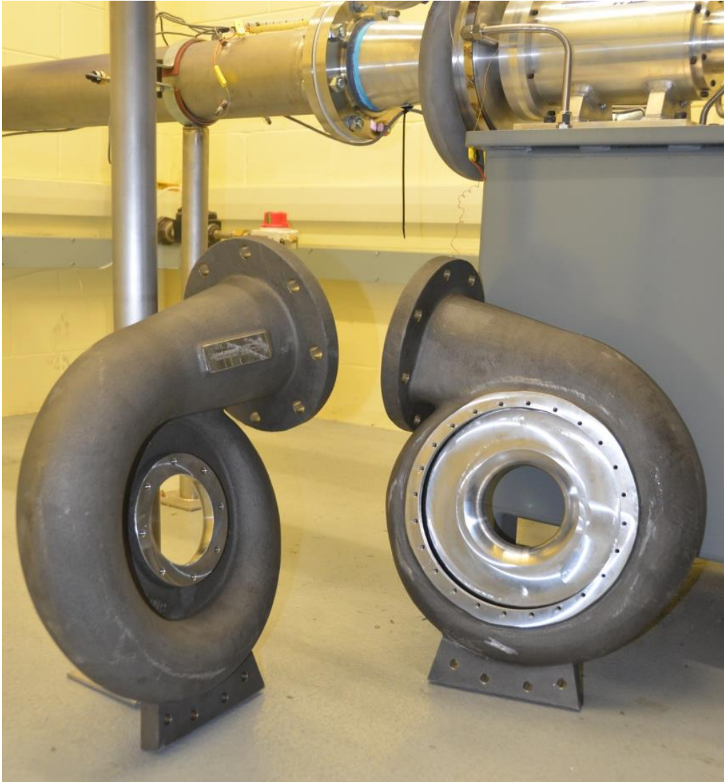
Figure 67. Stainless steel volutes for high pressure testing
