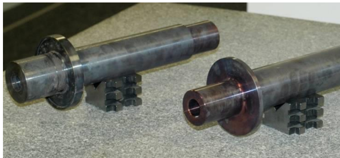
Figure 52. The two shafts of the dual-drive system of the single stage compressor. The rough shafts are shown following heat treatment (above). The shafts were then machined (above, right) and finally precision ground for a high-tolerance fit (right) with the motor assembly
