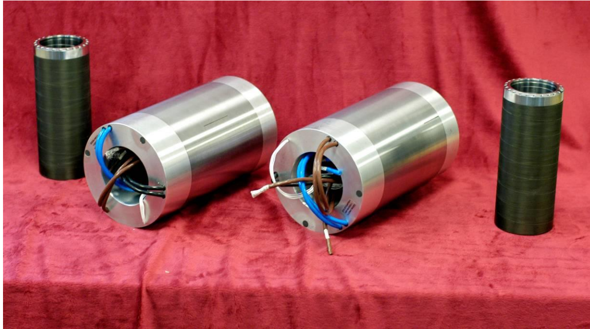
Figure 51. Pair of 100 kW motor elements for use in the dual drive single stage compressor
