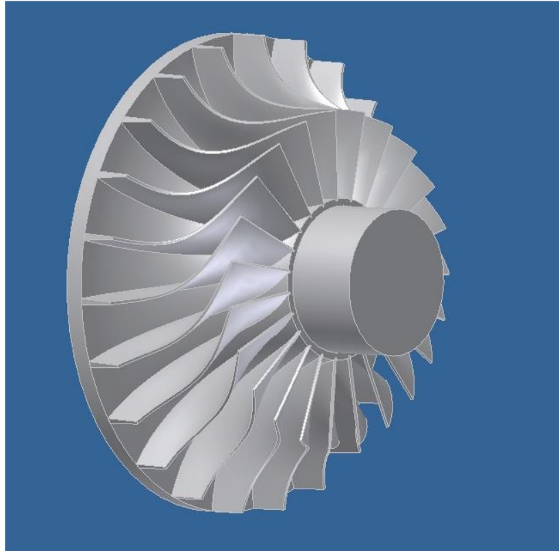
Figure 6. Preliminary geometry of the proposed single stage centrifugal compressor
