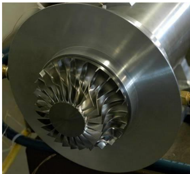
Figure 60. The bladed compressor wheel (left) and volute (right) attached to the 100 kW motor for performance testing.
