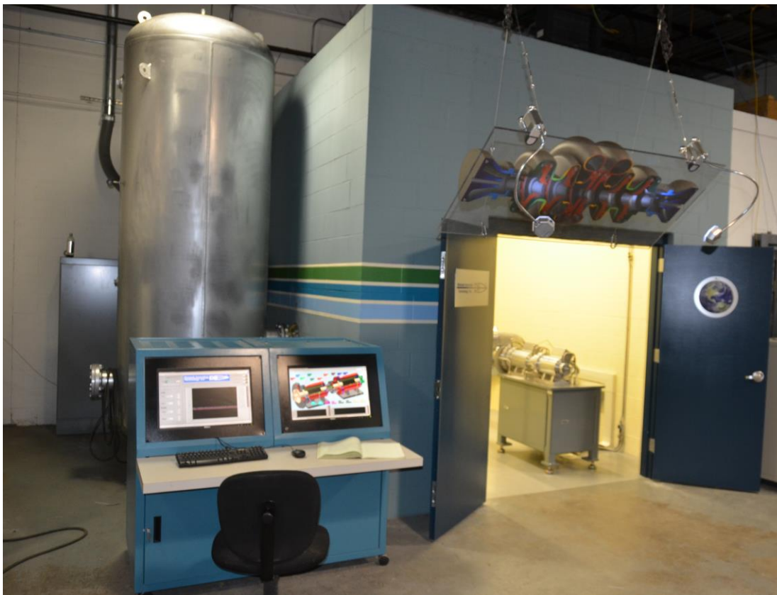
Figure 69. The instrumented single-stage compressor showing the test cell, the compressor, motor drive unit and command console
