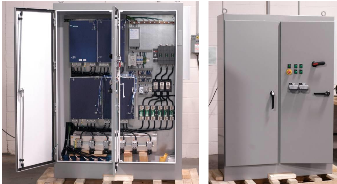
Figure 54. Dual motor variable frequency drives (VFD) shown after being received at MiTi
