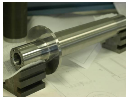
Figure 52. The two shafts of the dual-drive system of the single stage compressor. The rough shafts are shown following heat treatment (above). The shafts were then machined (above, right) and finally precision ground for a high-tolerance fit (right) with the motor assembly
