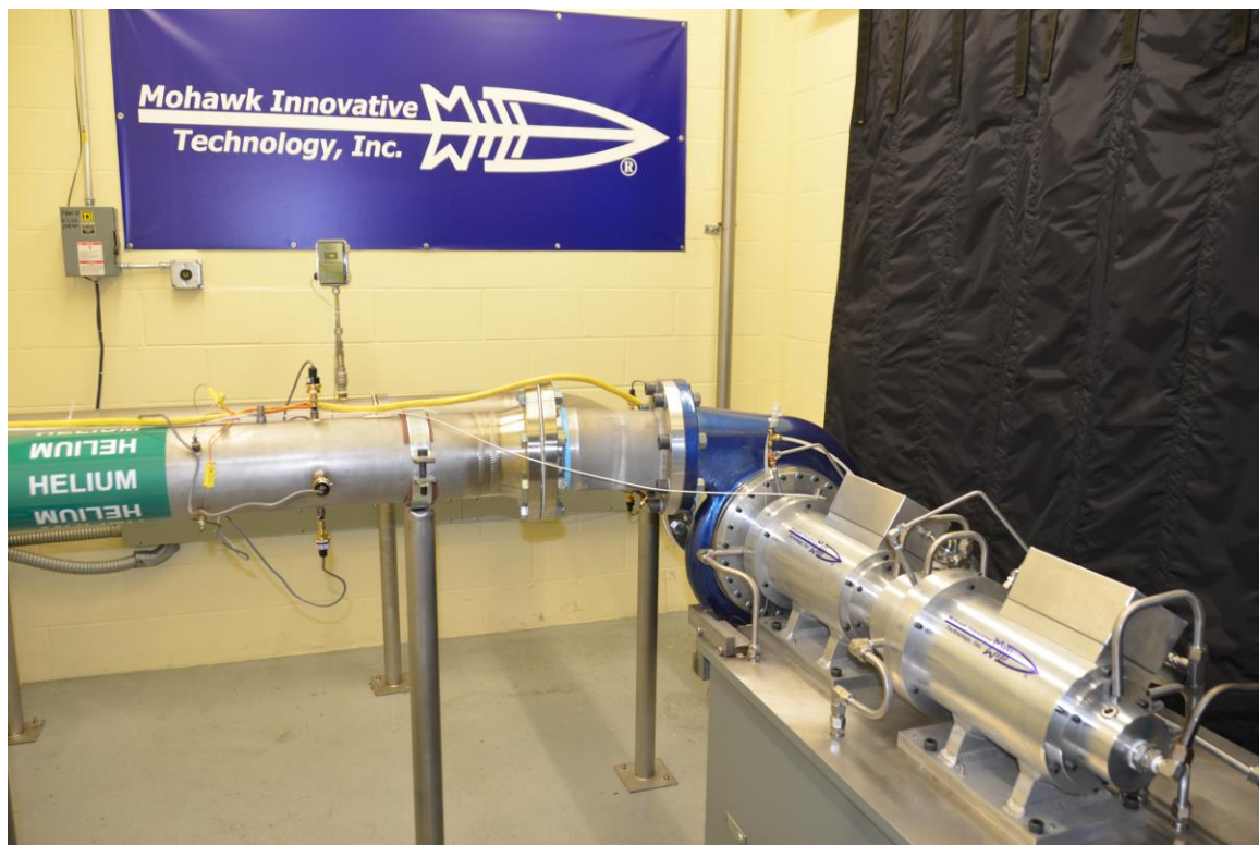
Figure 71. Single stage compressor with newly fitted stainless steel volute (blue in color) for higher ambient pressure testing
