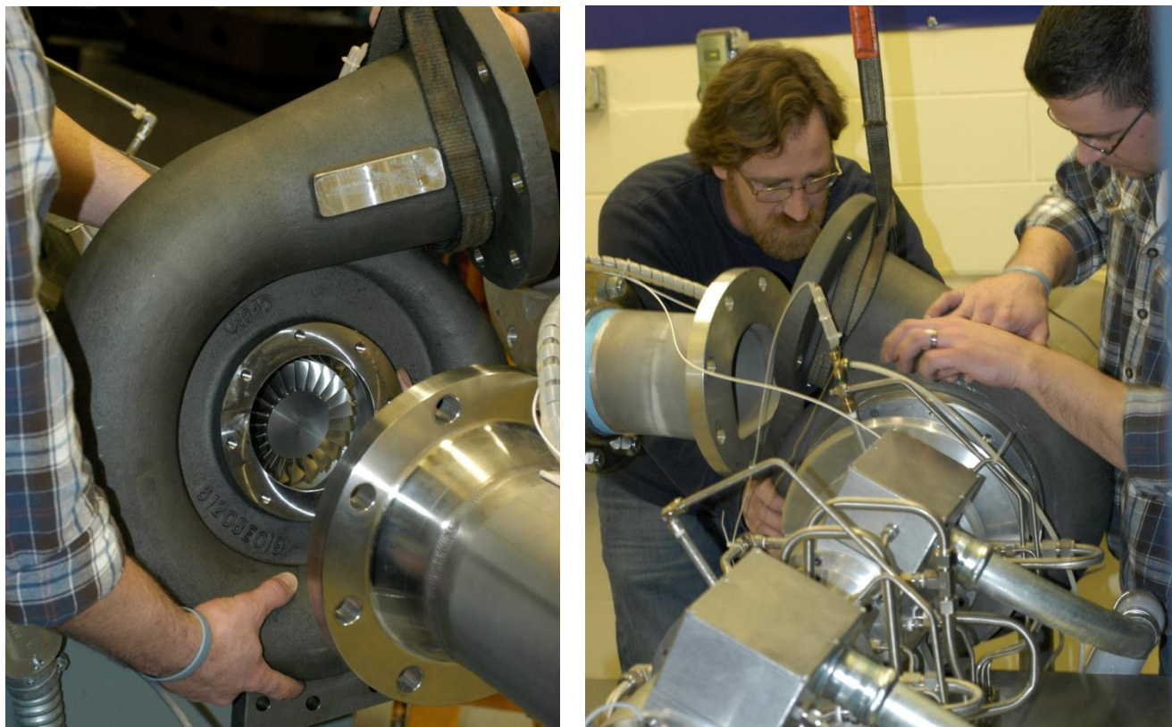
Figure 68. Fitting and installation of the stainless steel volute on the single-stage compressor
