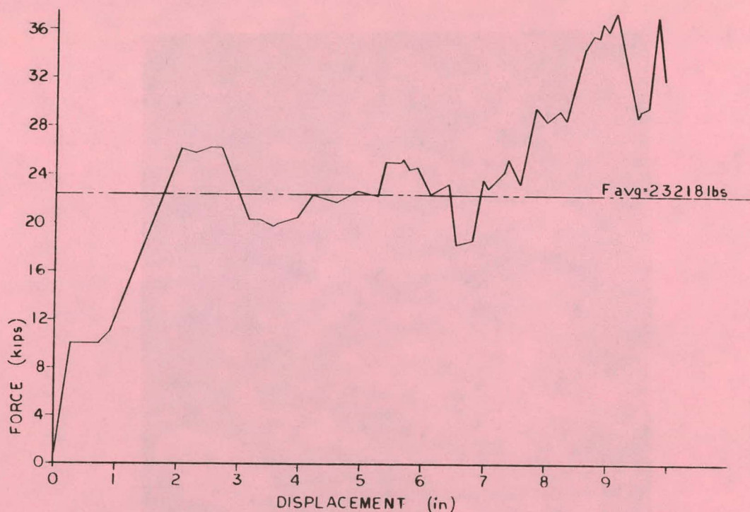
Figure 139. Half-Scale Front End Model 2 Energy Absorber Force vs Displacement
