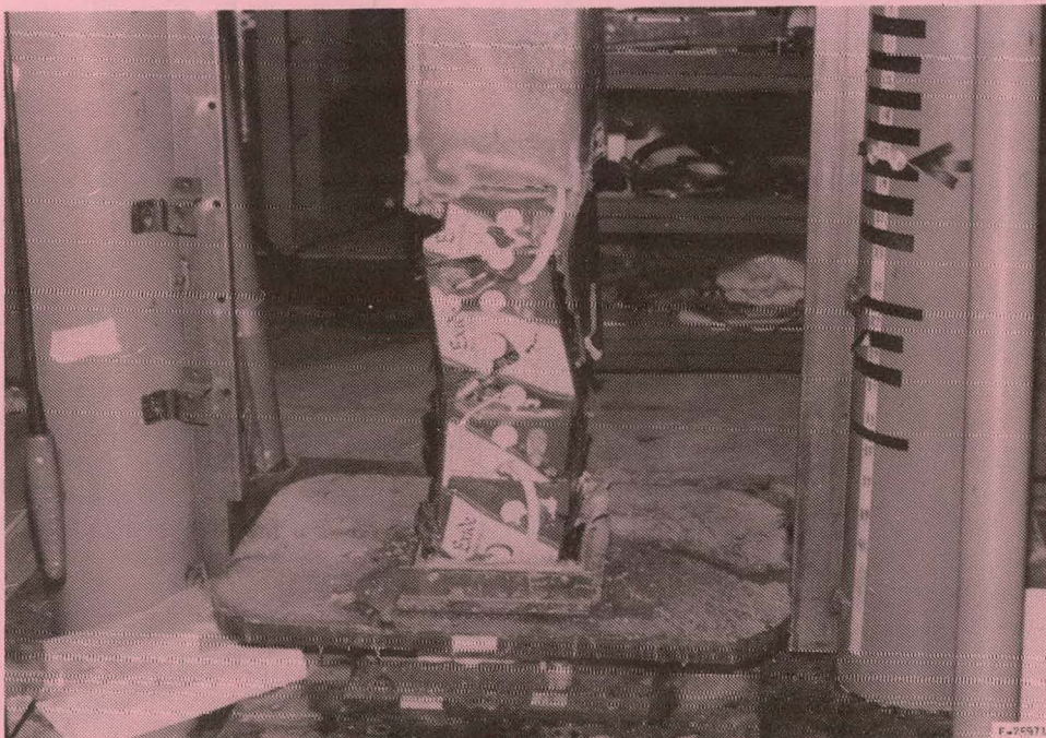
Figure 123. Battery Tunnel Crush Test Results
