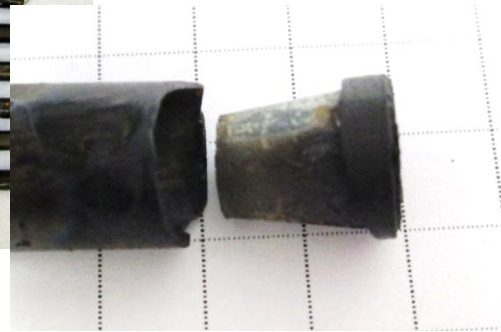
Fig. 3-28. Post-test fracture showing a primary failure in the joint with partial failure in the monolithic tube.
