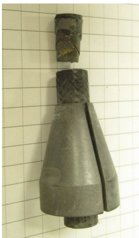
Fig. 3-56. Incusil joined composite tube post testing at 600 °C.
