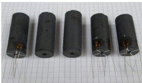
Fig. 3-31. EM 2 sized GA Hybrid joined test specimens with hole in endplug to vent fission products. Three of the specimens have been mounted with strain gauges.
