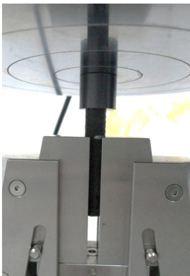
Fig. 3-7 (left). Mechanical test of maximum applied load for active gripping.
