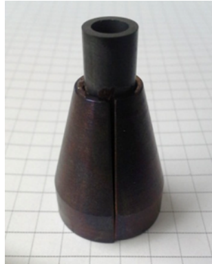
Fig. 3-5. Bonded monolithic tube to stainless steel collets using Morgan Incusil Braze.
