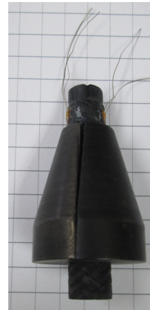
Fig. 3-12. Specimen ready for testing with strain gauges and collet installed.
