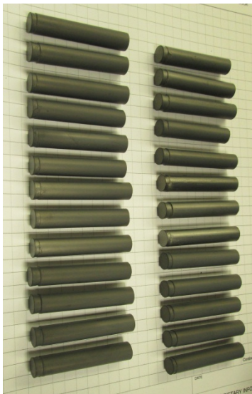
Fig. 3-58 (Left). A set of 26 monolithic SiC Tube, CD SiC Endplug, and GA-HSiC joint specimens awaiting high temperature testing.
