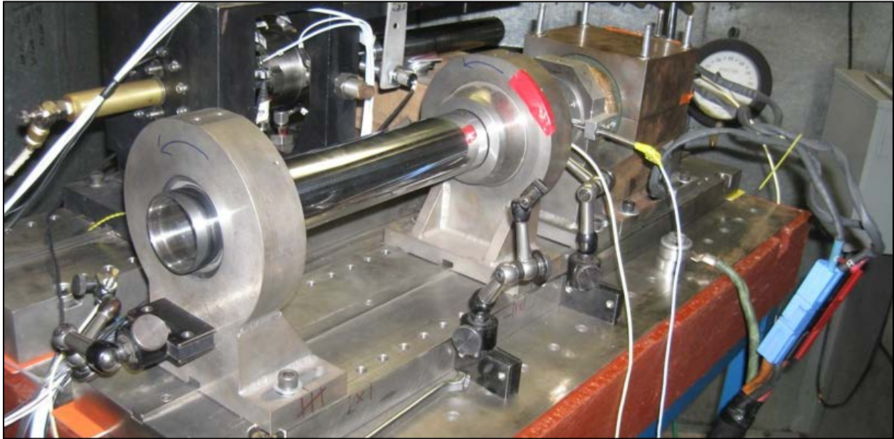
Figure 21: Generator Shaft Rotor dynamics Test Rig
