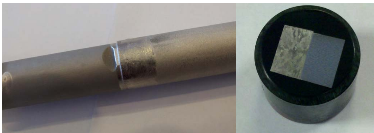
Figure 84: Finished Tensile Sample and Sample Mount Showing Material Differences
