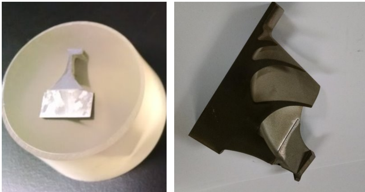
Figure 87: Tensile and Micrograph Analysis of One of the Bonded Prototype C65 Turbines
