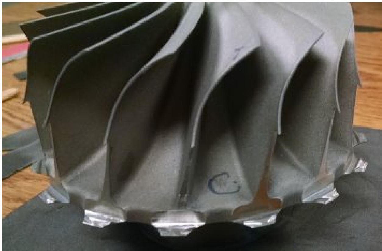
Figure 81: C65 Turbine with Blade Tips Removed
