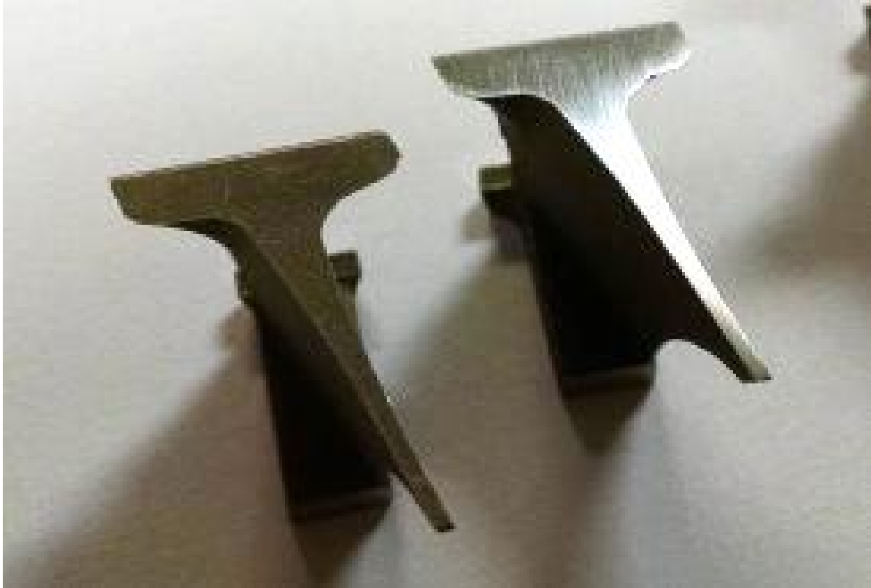
Figure 82: Single Crystal Tips for Prototype C65 Turbine wheel
