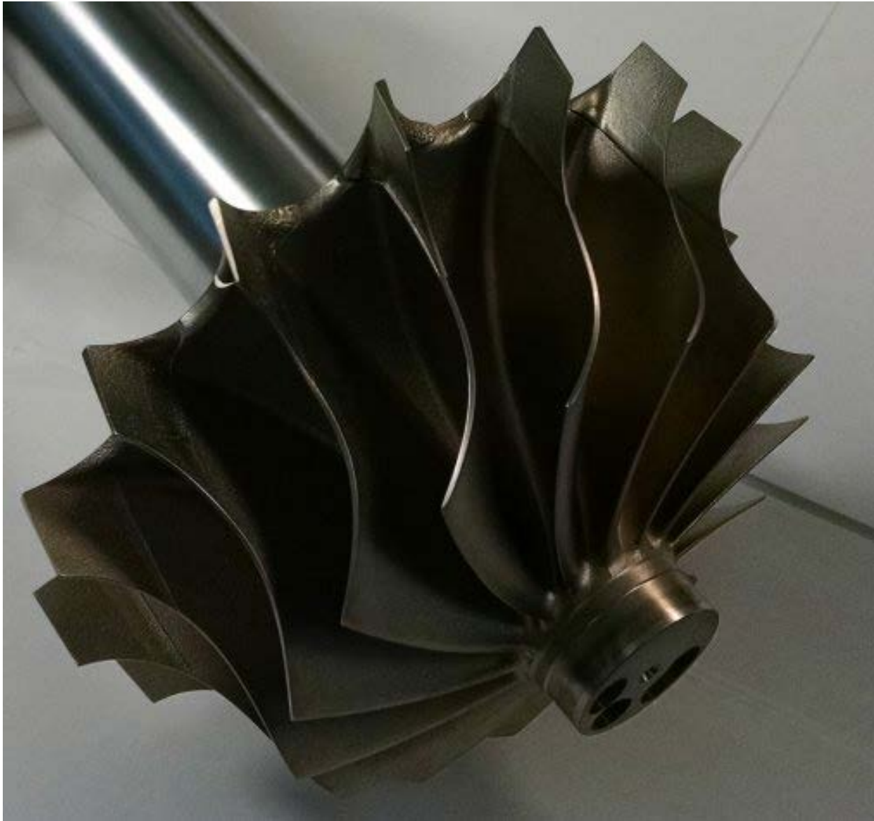
Figure 74: C65 Prototype of a Bi-Metallic Turbine Wheel
