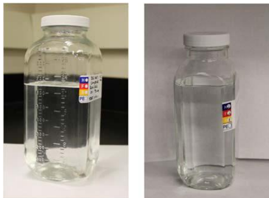
Figure 12. Solid wax-free clear hydrocarbon liquids produced by Chevron catalyst
