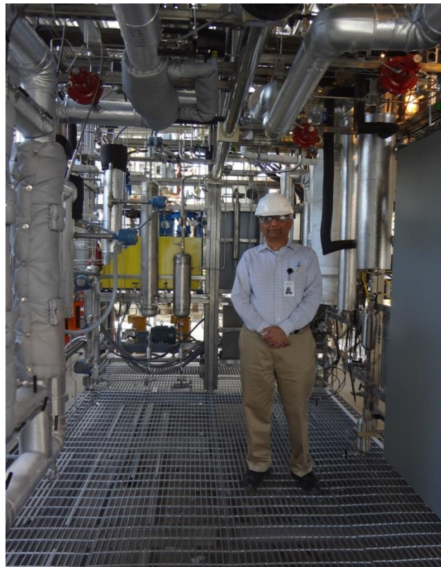
Figure 5. SR-CBTL test-rig in position at NCCC; walk-in and around capability; Hot sulfur trap on left; Purged PLC Enclosure on Right
