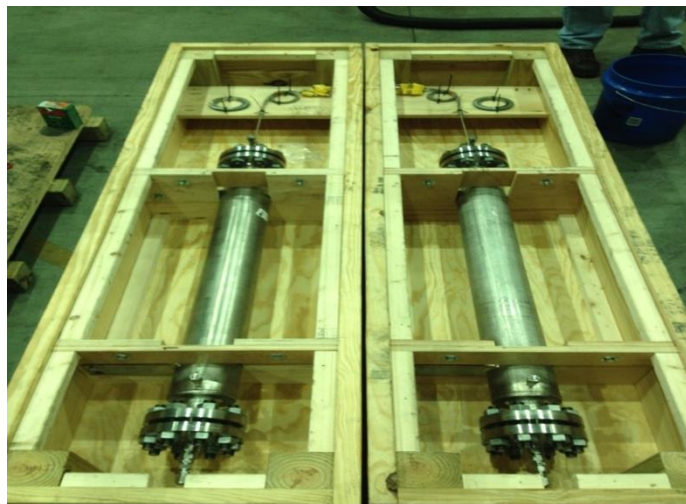
Figure 10. Jacketed 2 inch diameter FT reactors with six position thermowell
