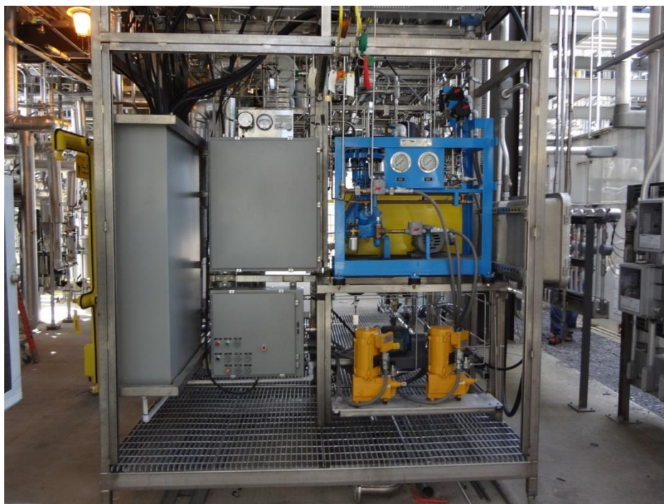
Figure 8. Rear view; compressor, mass flow controller panel, power panel, scrubber water pumps
