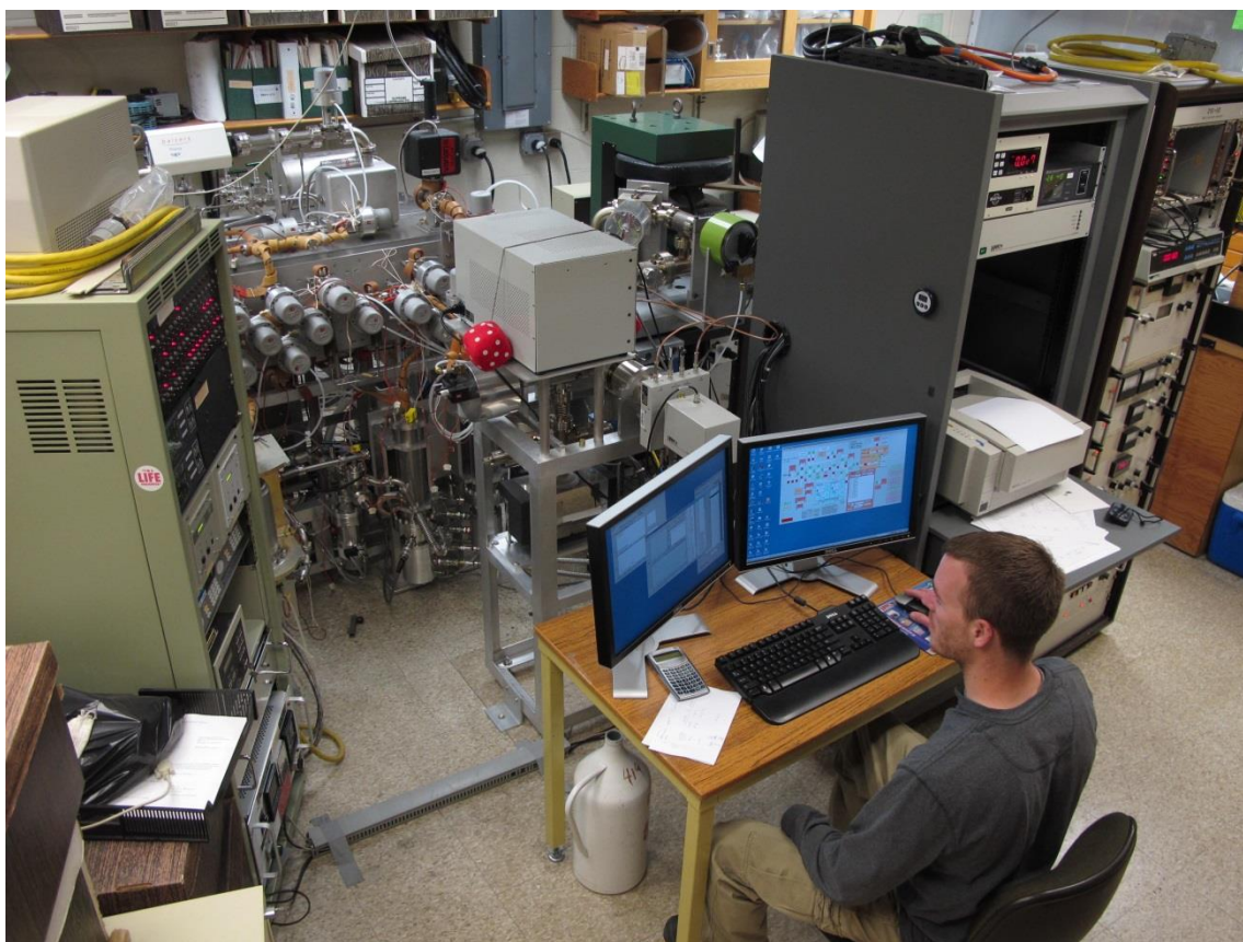
Figure 2. MAP 215-50 Mass spectrometer used to measure helium, neon, and argon at Woods Hole Oceanographic Institution (WHOI). The extraction line shown in figure 1 was designed to pre-purify samples for transfer to this system, thus avoiding hydrocarbon contamination. Samples are transferred to this system using stainless steel containers.
