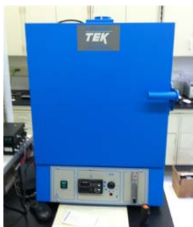
Figure 2. Furnace used to thermal age XLPE nanocomposites at a temperature of 120°C.
