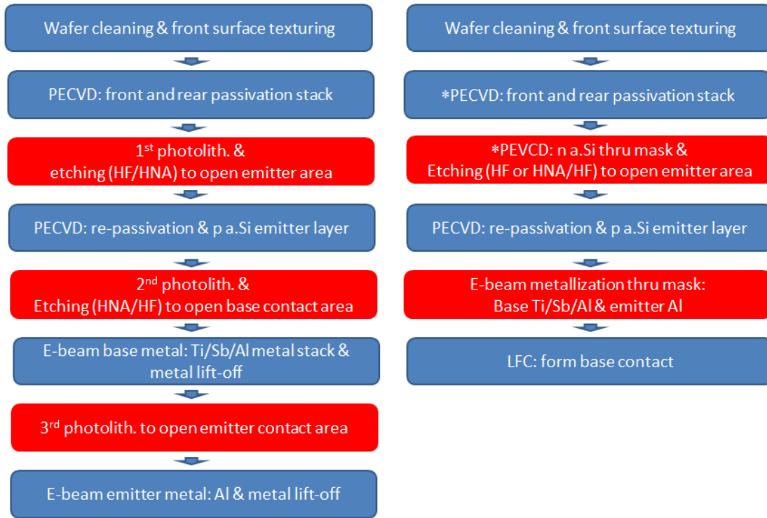
Figure 10.3. Process flow for the 2 different patterning processes: a) 3-step PL; b) masked deposition (MD)
