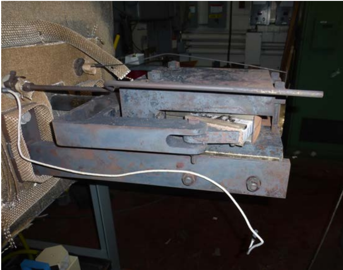
Figure B-2: HV Wire Clip Failure
