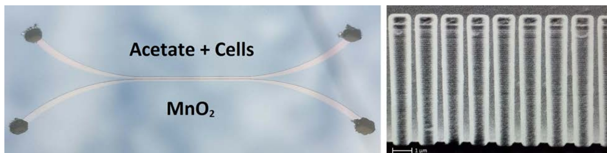
Figure 3: A picture of the microfluidic reactor (left) showing experimental conditions, and an SEM image of the physical barrier (right) that separates the center region where the two channels meet.
