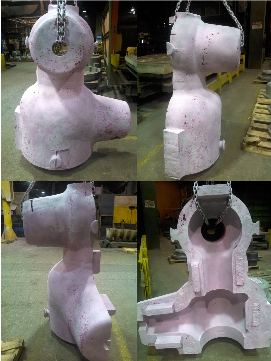
Figure 104: Haynes 282 Valve casing Liquid penetrant testing 100% surface area
