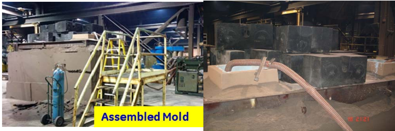
Figure 95: Assembled mold, hot air dried and purged with Argon prior to pouring [Courtesy-MetalTek MO]
