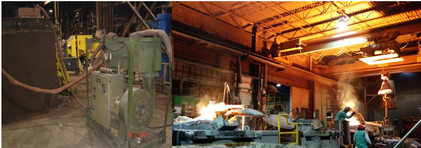
Figure 96: Induction melted, composition controlled with argon cover during melting and tapping melt quality controlled [Courtesy-MetalTek MO]
