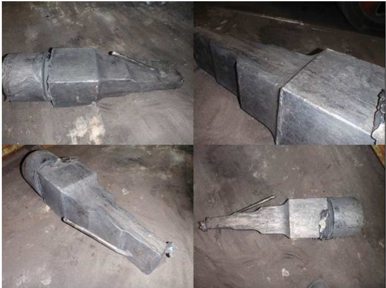
Figure 19: MetalTek 300 lbs. Haynes 282 step block casting after mold shake out and shot blast cleaning operations. Bottom gated with casting top feeder arrangement shown.
