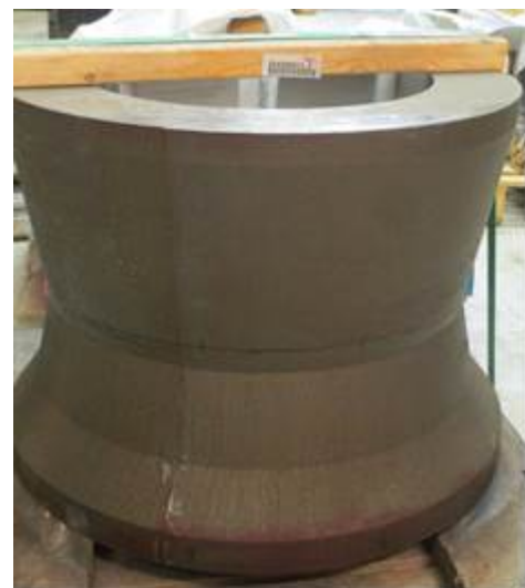
Figure 60: Picture showing the extraction of the slice for heat treatment and micro-structural analysis
