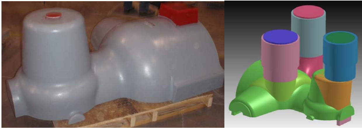
Figure 91: Foundry Casting Pattern and feeder design
