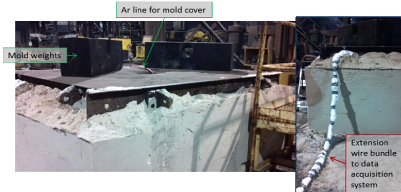
Figure 83: Photograph of completed mold ready for pour
