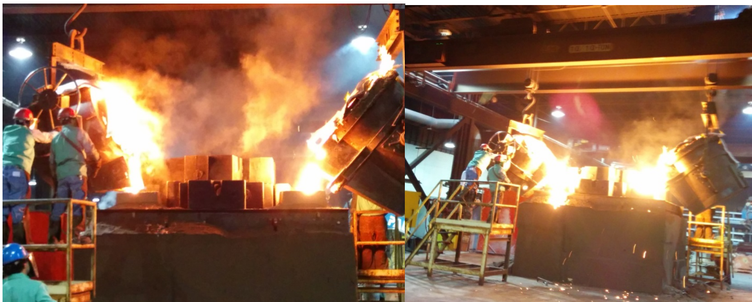
Figure 97: Pouring the mold after deslagging with covered ladles ensuring targeted pouring temperature and pour times
