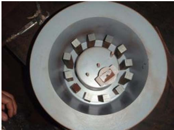
Figure 79: Photograph of chills location in mold pattern prior to molding
