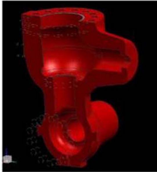
Figure 90: Steam turbine half valve casing selected for the large casting trial
