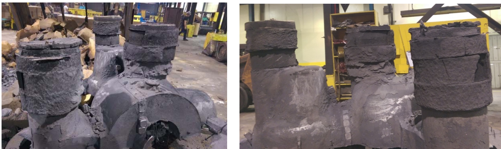
Figure 98: Casting after in mold cooling and shake out [Courtesy-MetalTek MO]
