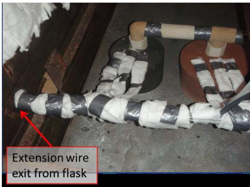
Figure 81: Photograph of thermocouple compensating cables routing within the drag mold
