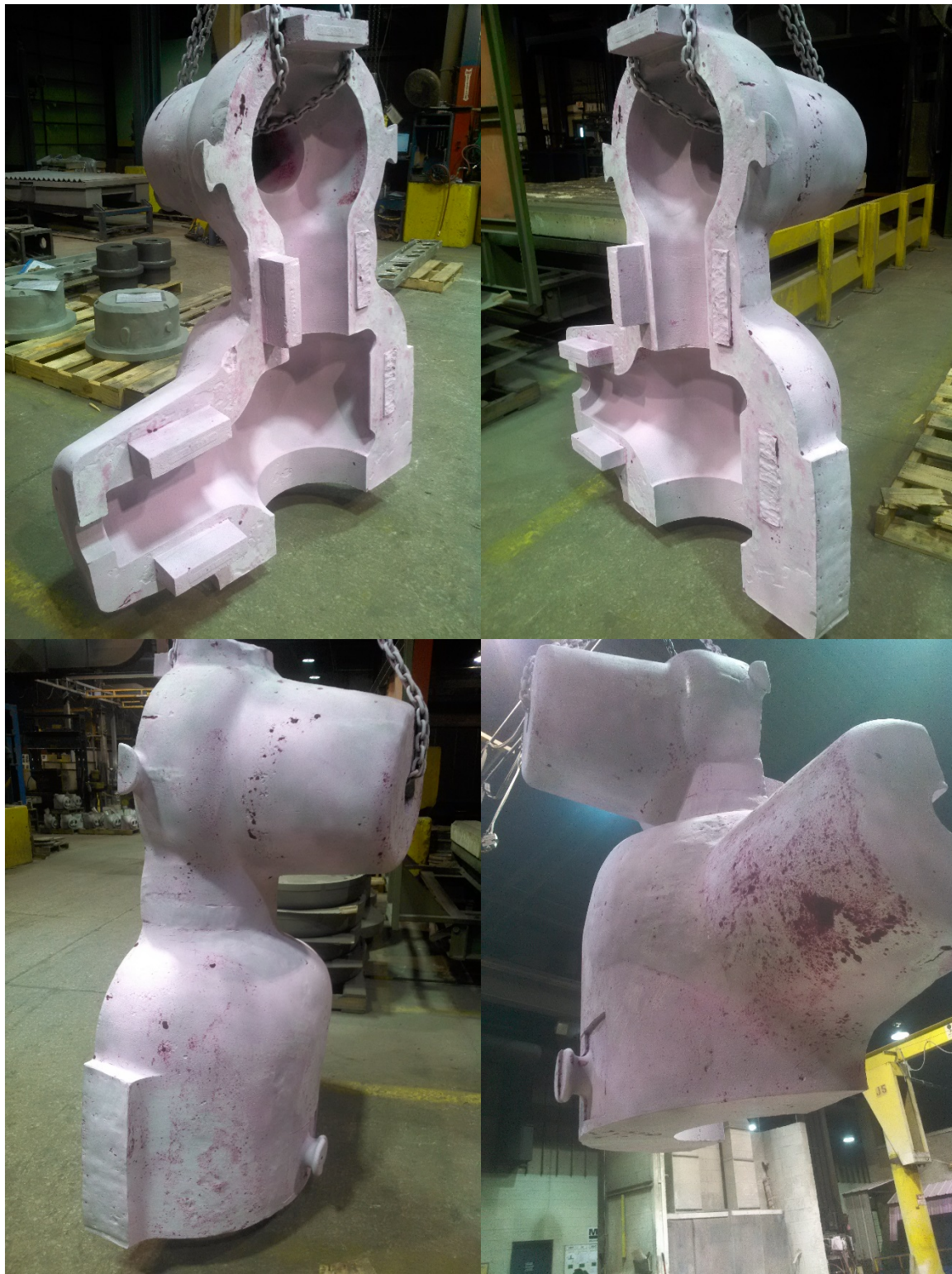
Figure 105: LPT inspection pictures on 100 % Cast surface areas
