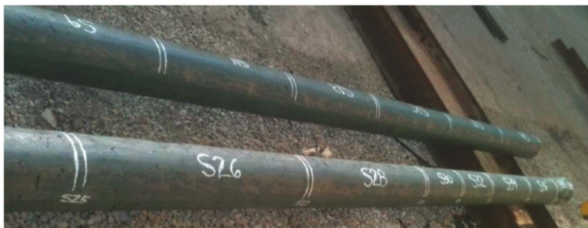
Figure 39: EX0045PW was forged into 8" diameter for macro-segregation evaluation
