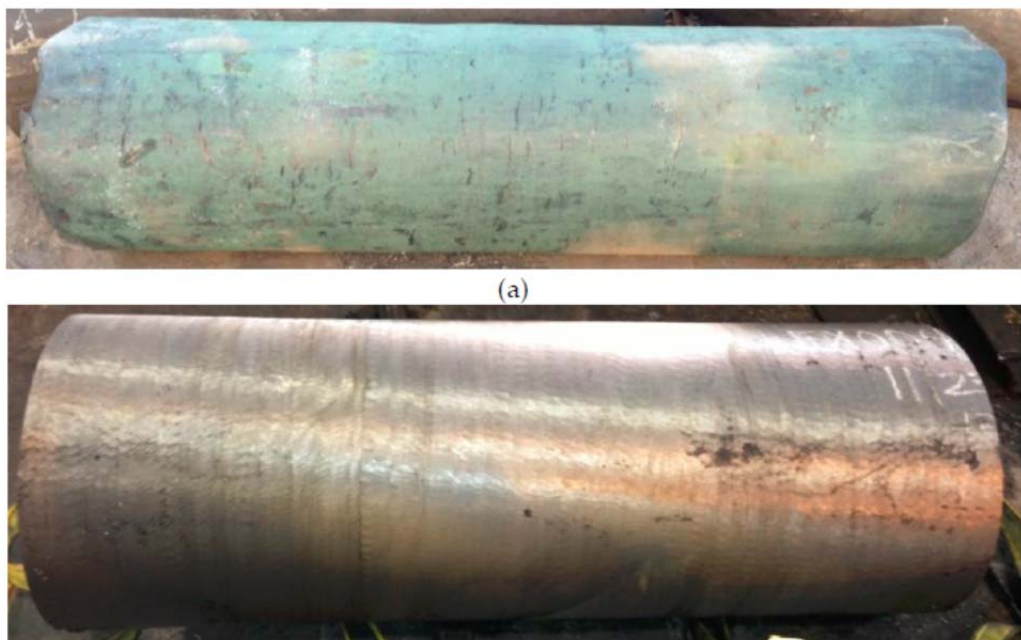
Figure 42 Second ingot EX0046PW billetized in (a) as forged condition and (b) after surface grinding to final diameter
