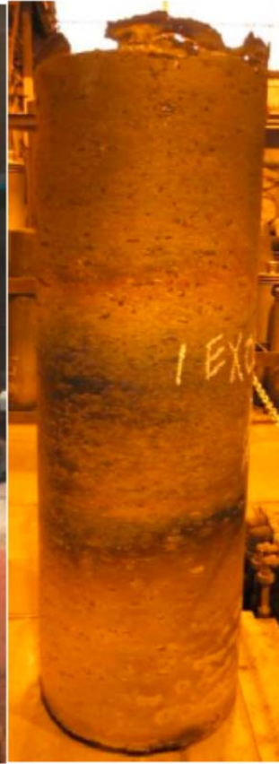
Figure 36: Pictures showing the 18" VIM / 22" ESR and the final 24" VAR Ingot.
