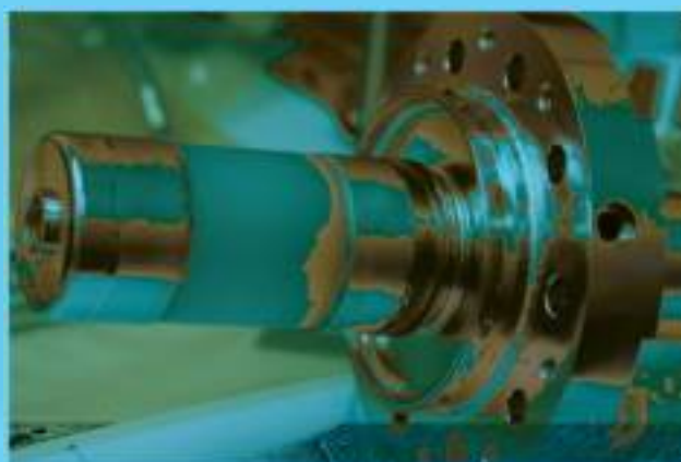
Figure 4: Sapphire Window brazed on to Niobium cuffs.
