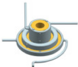
Figure 6: Original Filter Assembly attached with Stycast (above) and new concept (below)
