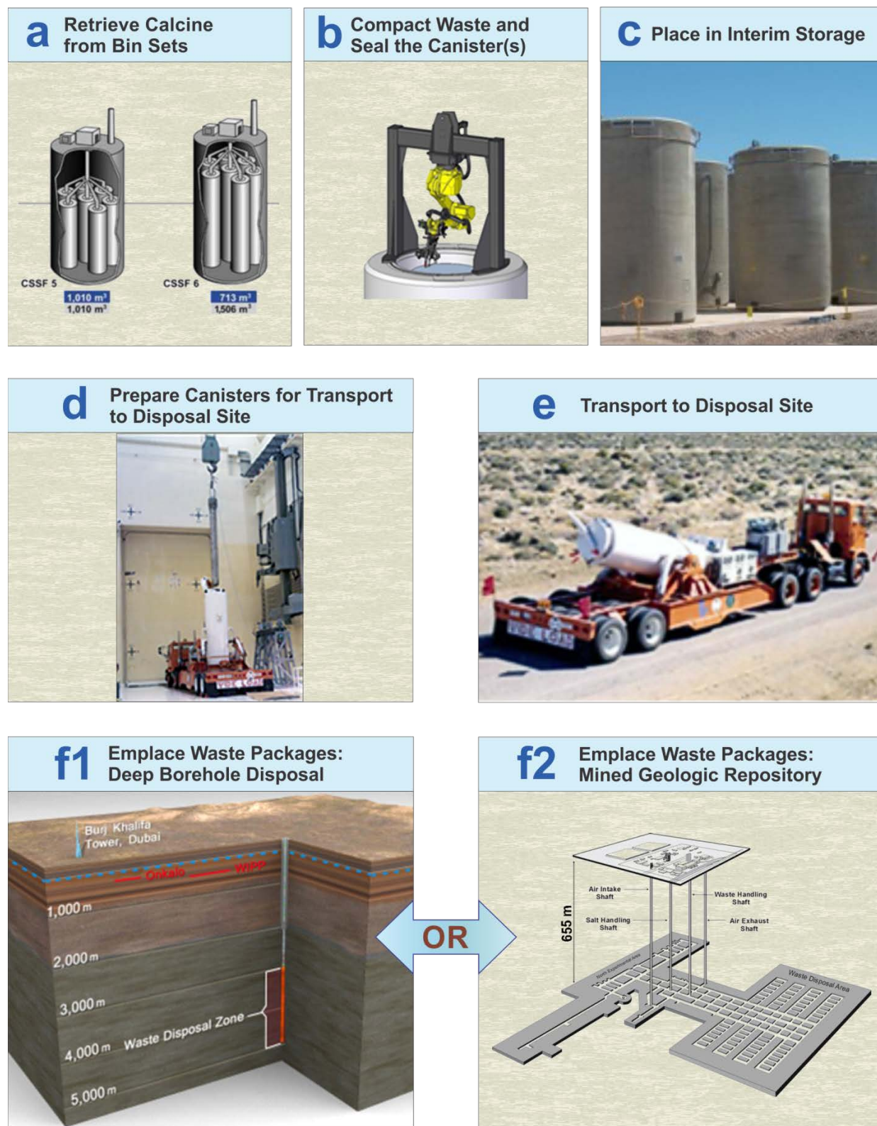
Figure 5-2. System Concept for Disposal of Calcine Waste in a Deep Borehole or Mined Geologic Repository
