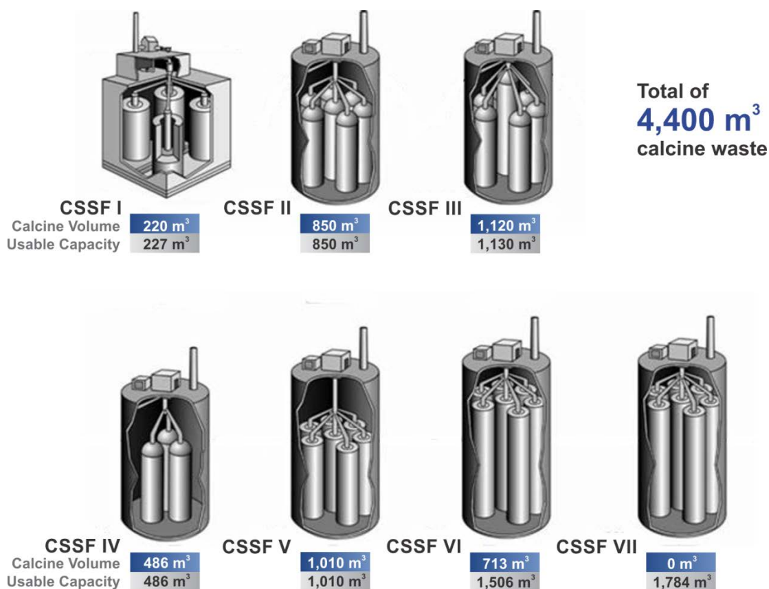
Figure 4-6. Cutaways of Each of the Seven CSSFs
