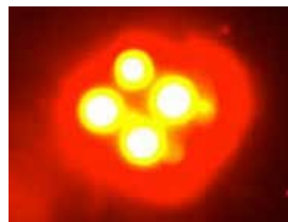
Images of 2x2 microscale discharge devices containing (from left to right) helium, argon, and neon. Images are looking down into cavities each 100 \mu\text{m} in diameter. Dielectric separators are 10 \mu\text{m} long.
