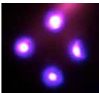
Images of 2x2 microscale discharge devices containing (from left to right) helium, argon, and neon. Images are looking down into cavities each 100 \mu\text{m} in diameter. Dielectric separators are 10 \mu\text{m} long.
