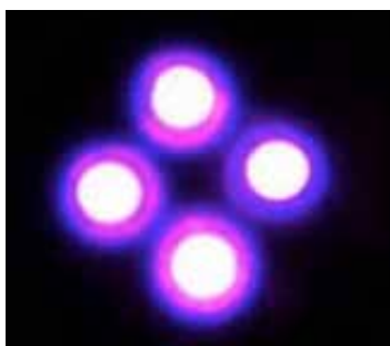
Images of 2x2 microscale discharge devices containing (from left to right) helium, argon, and neon. Images are looking down into cavities each 100 \mu\text{m} in diameter. Dielectric separators are 10 \mu\text{m} long.
