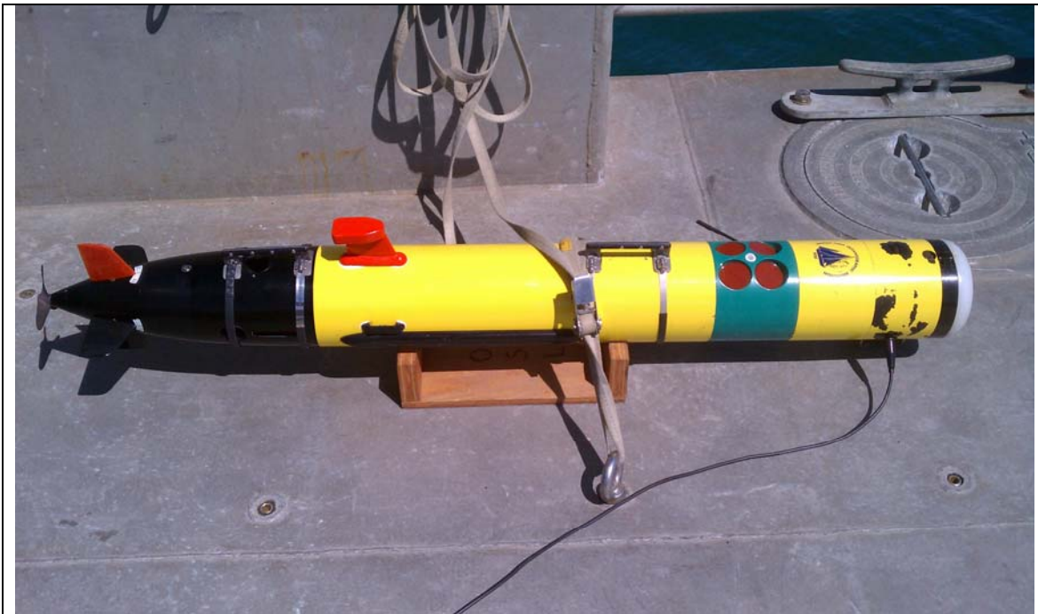
Figure 9. WHOI OSL REMUS. The green module is an upward/downward-facing 1200 kHz ADCP. The orange “fin” is a GPS antenna used for navigation.
