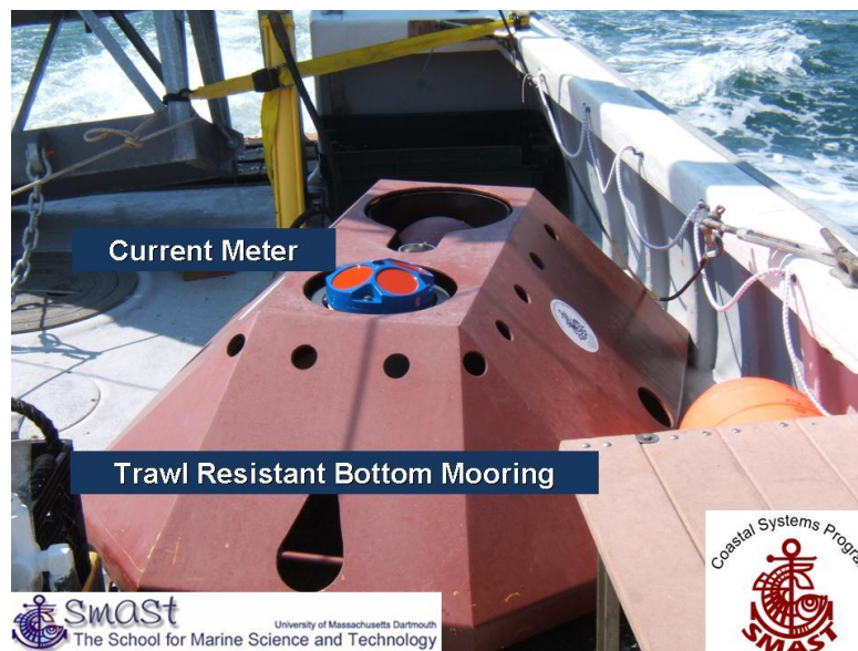
Figure 6 – ADCP deployed November 2010 to measure current velocity over a complete lunar cycle in the high velocity zone of Muskeget Channel.
