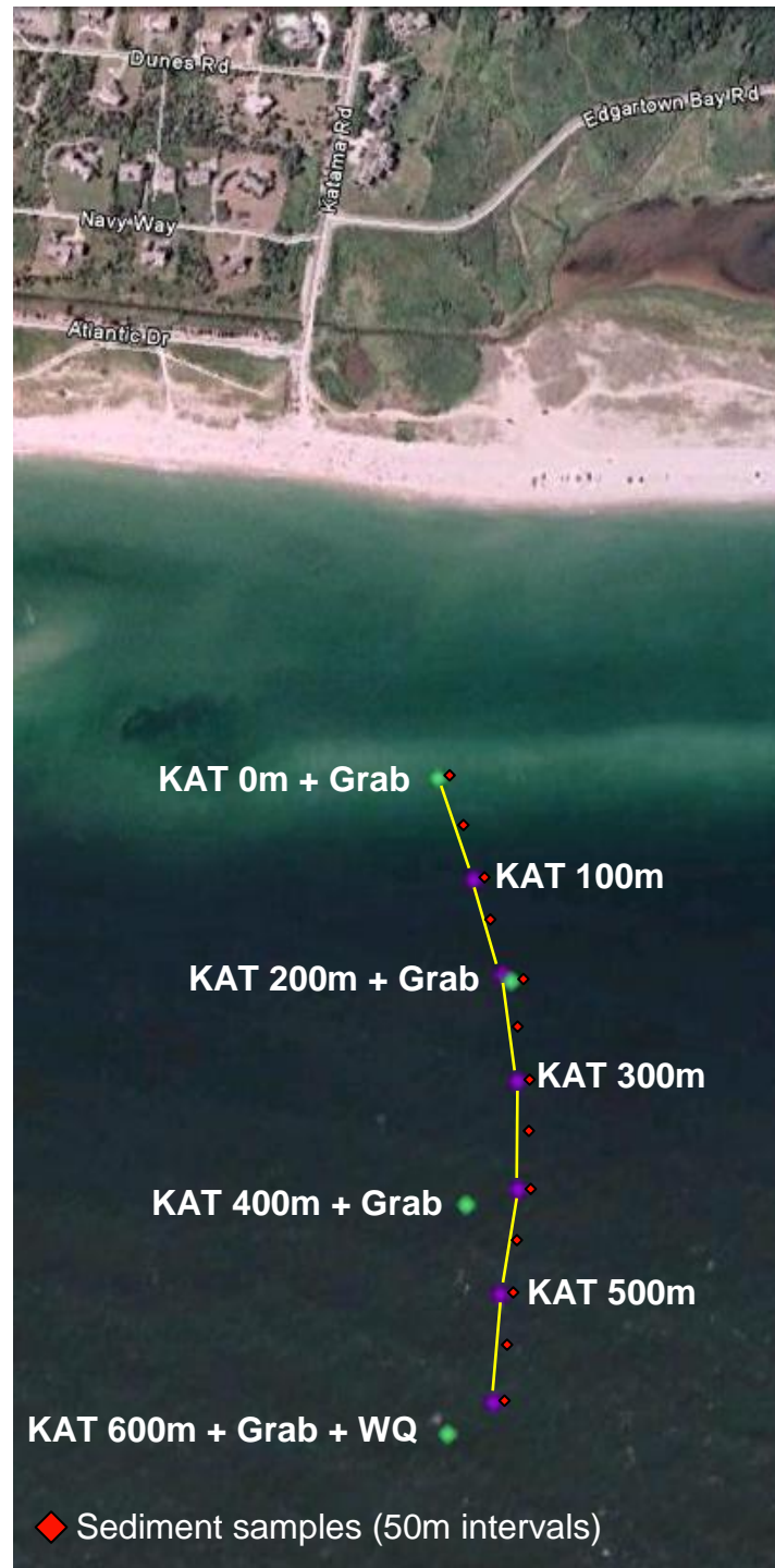
Figure 31 – Katama Transect, Martha's Vineyard south shore. Infaunal grab samples retrieved at 200 meter intervals (green symbols) with associated disturbance plots. Sediment samples retrieved at 50 meter intervals (red symbols). Underwater surveying completed by diver observation for eelgrass and bottom characteristics the length of transect.
