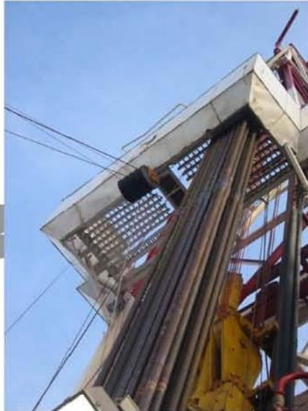
1. Example of the common position of the sheave wheel hanging in the derrick
