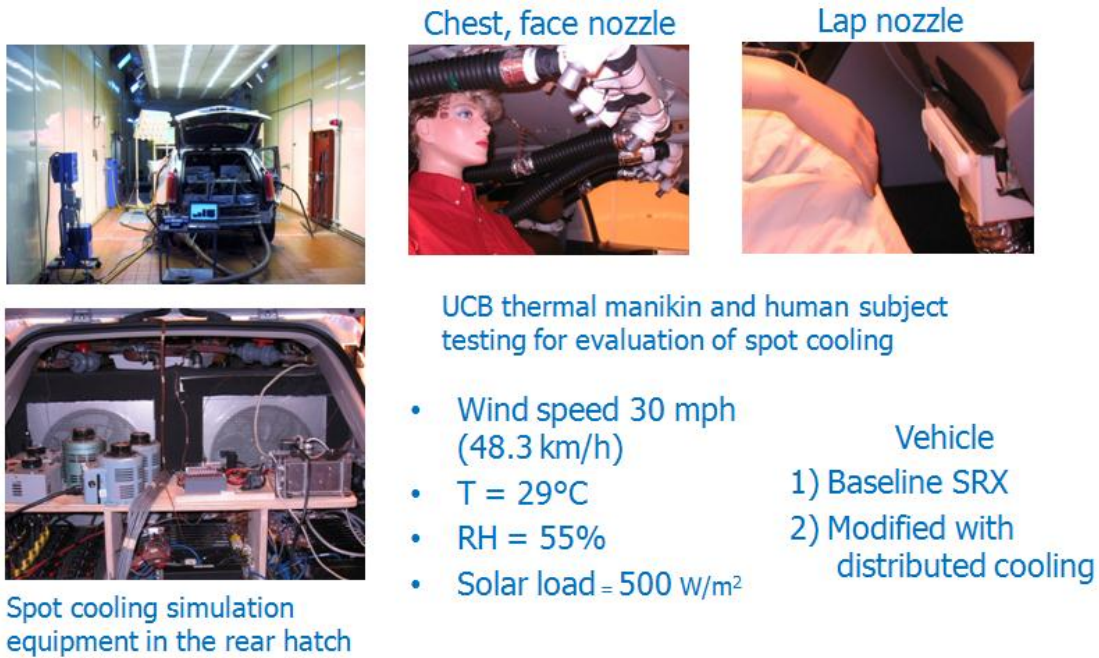
Figure G12: Thermal comfort validation setup for the baseline spot cooling case
