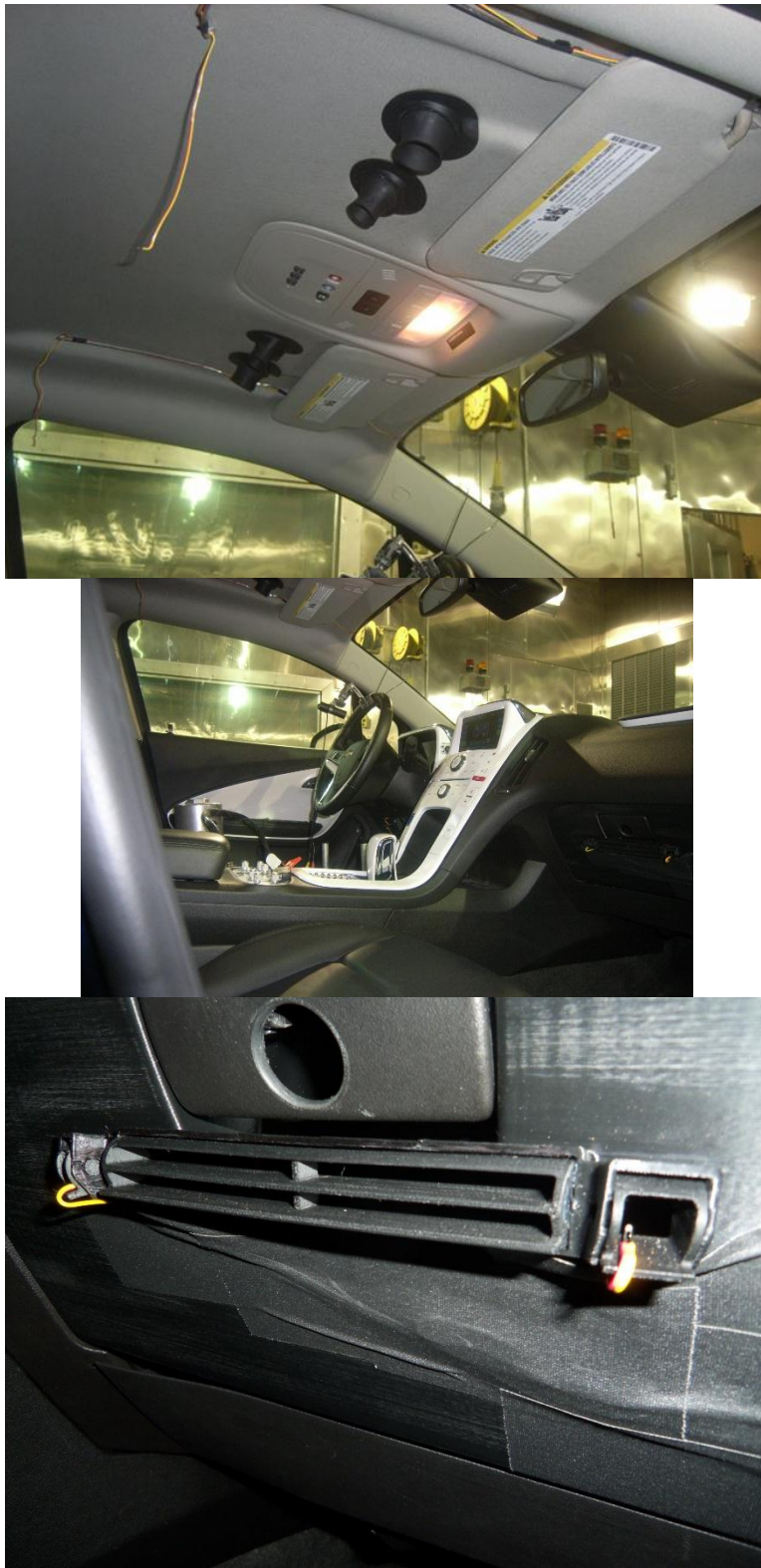
(a). Chest-Face nozzle, (b) TE seats, (c) Front passenger lap slot nozzle
