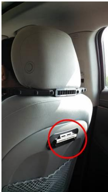
(a) Lap TE slot nozzle on the front passenger side
