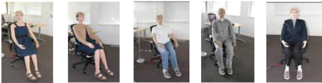
Figure G5: Measuring insulation levels for 16 body parts in typical clothing ensembles
