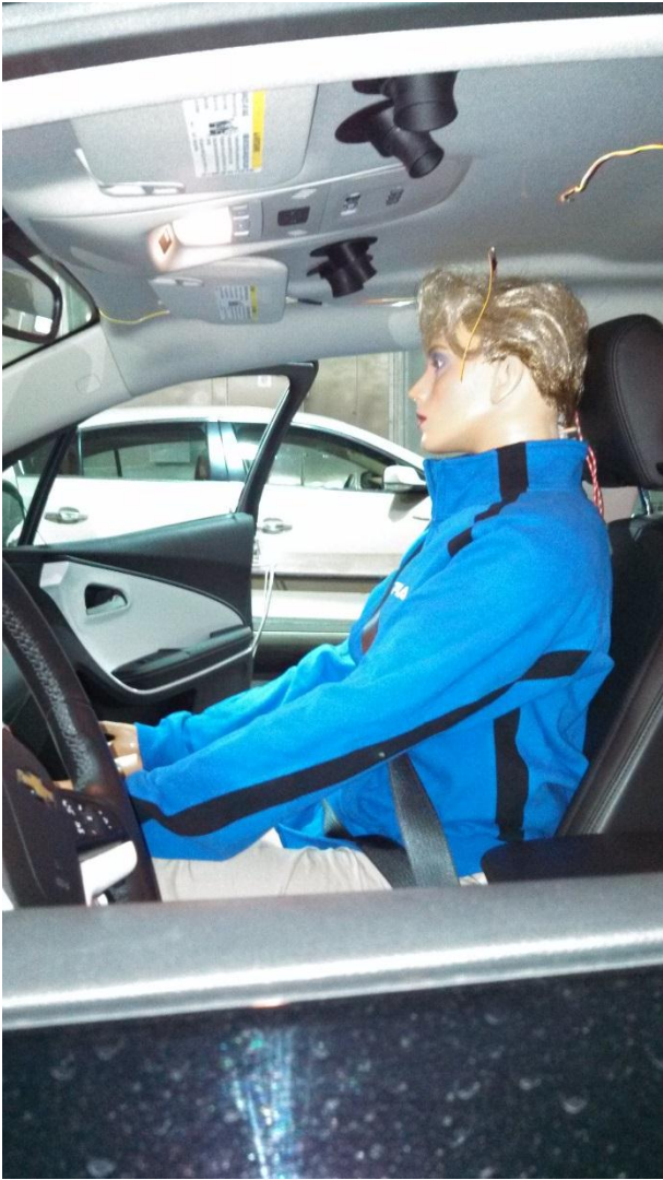
Figure G112: The thermal manikin, Monika, is positioned in the front passenger seat
