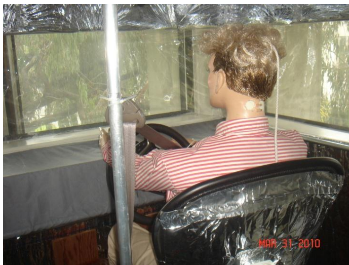
Figure G25: A thermal manikin is used to measure the heat loss of various local cooling/heating devices
