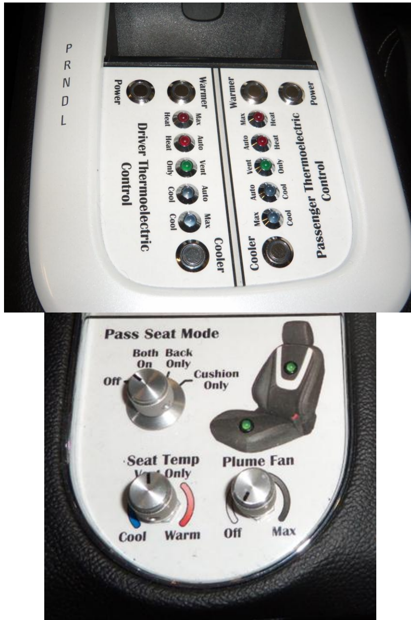
(d). TE HMI control for Chest-Face nozzles, (e) TE HMI control for front seats
