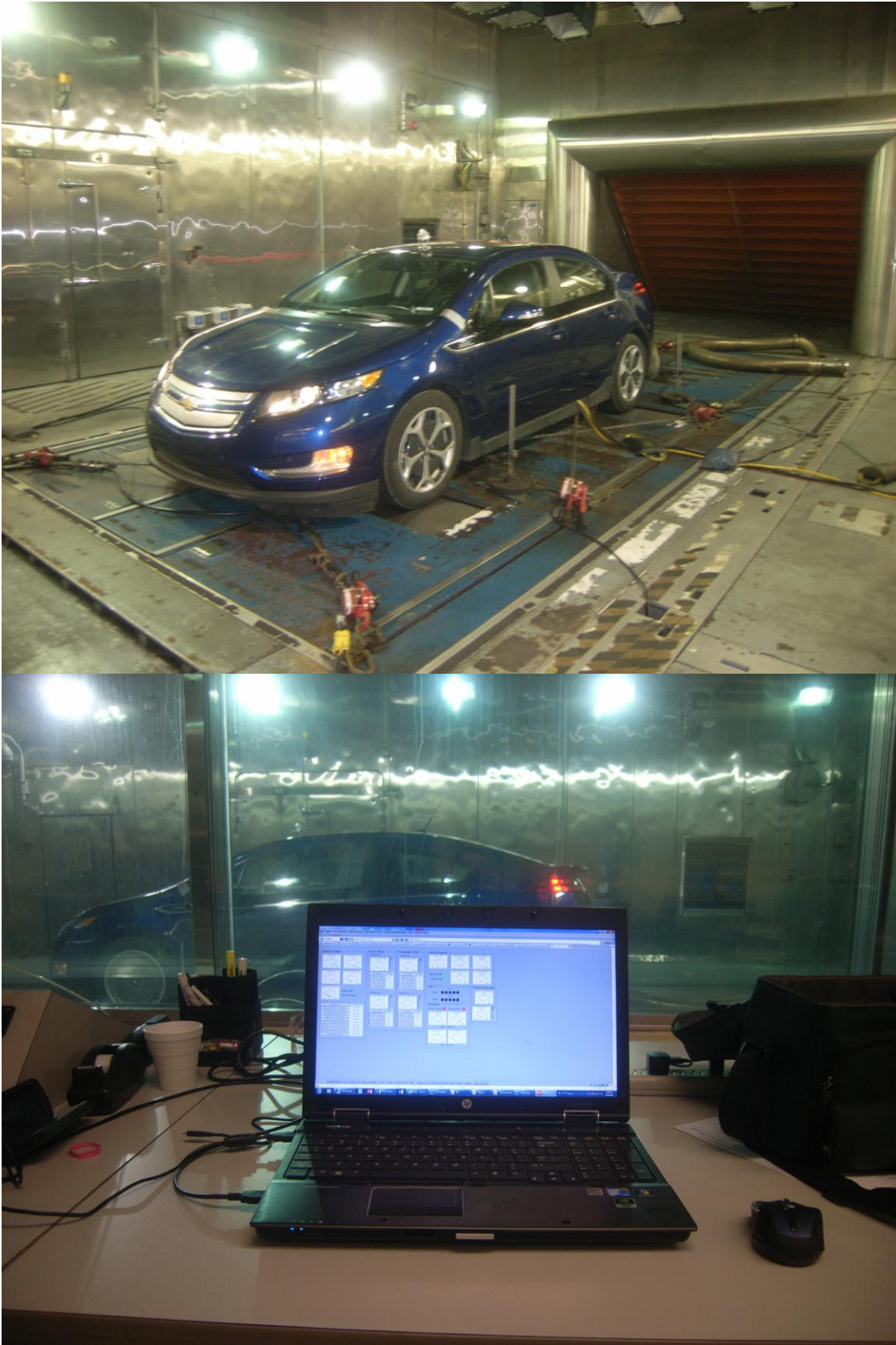
Figure G111: The Volt in GM's Climate Wind Tunnel and data collection in the control room
