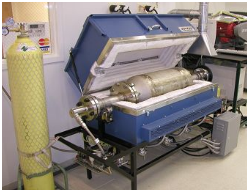
Figure 2. Rotary furnace for 1 cu ft. batch size.
