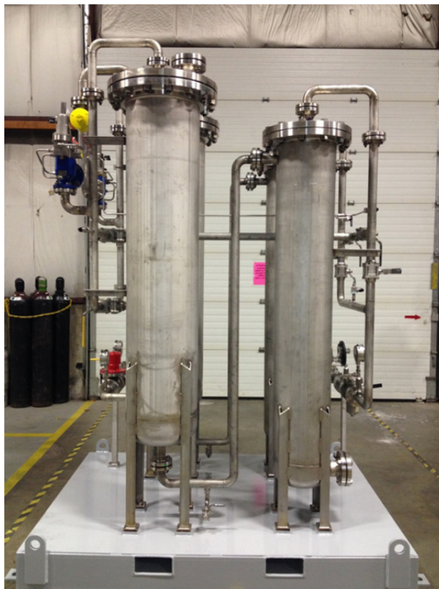
Figure 41. Picture of lead-lag full-scale prototype skid.
