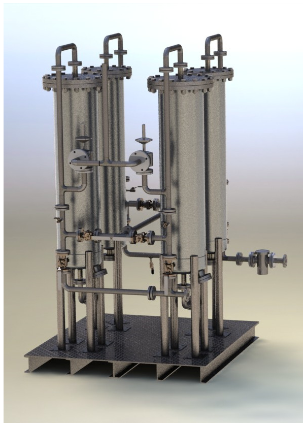
Figure 40. 3-D layout of the lead-lag prototype desulfurizer skid
