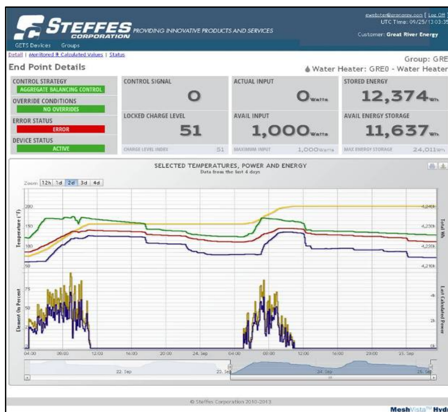
Figure 13.8: Steffes Data on Temperature, Power, and Energy for an Individual Water Heater
